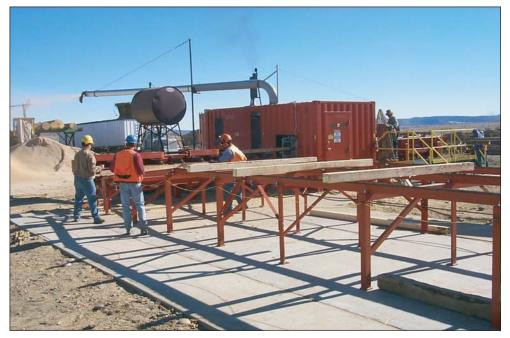
Figure 9—MicroMill outfeed after sawing small-diameter logs in Flagstaff, Arizona. (The use of trade or firm names is for reader information and does not imply endorcement by the U.S. Department of Agriculture of any product or service.)
