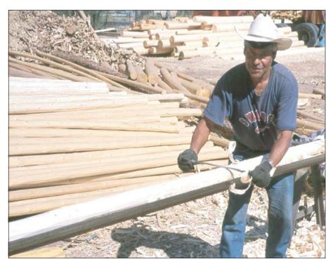
Figure 7—Hand peeling bark for exposed ponderosa pine latillas in Arizona.
