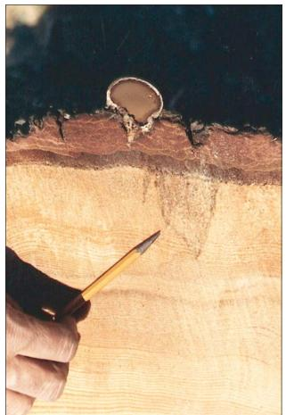
Figure 4—Decay fungi fruiting body and sap rot in Douglas-fir log 2 years after fire kill.
