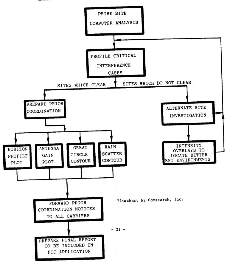
The rules contain no prescribed method of calculating interference between terrestrial systems. However standard procedures and models have evolved in the industry and have been incorporated in the various proprietary computer programs utilized by the companies who perform such calculations. The need for a greater degree of standardization in these computational programs is one of the issues being studied by the NSMA.
