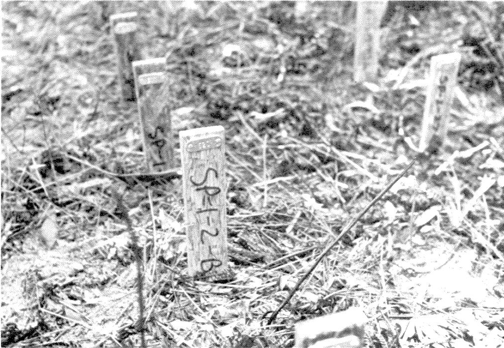
Figure 3.--Composite wood decay stakes in Florida test plot, used for ground contact evaluation.
