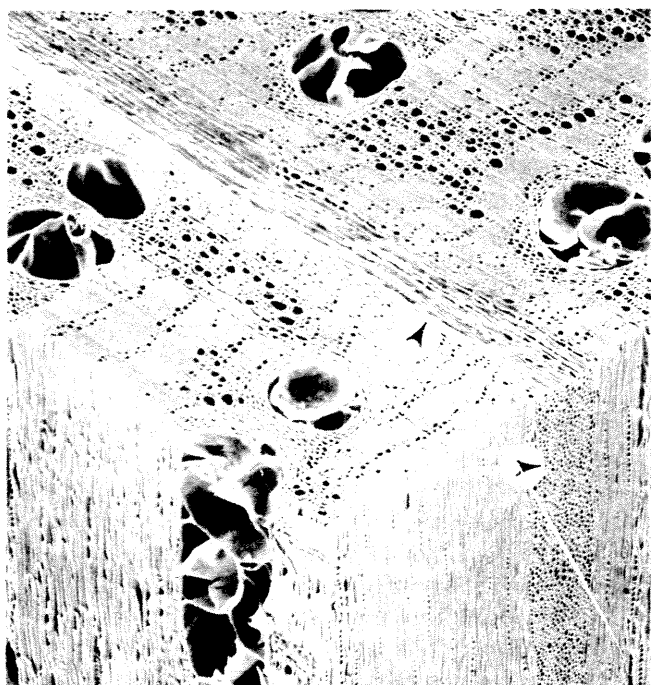
Figure 6.—Scanning electron micrograph of large rays in hardwood.
