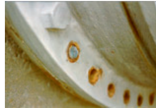
Figure 3. Dezincification of Brass Containing a High Zinc Content.[4]
