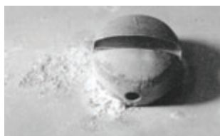
Figure 2. Galvanic Corrosion between a Stainless Steel Screw and Aluminum. A Cathodic Material for Fasteners is Preferred.[2].
