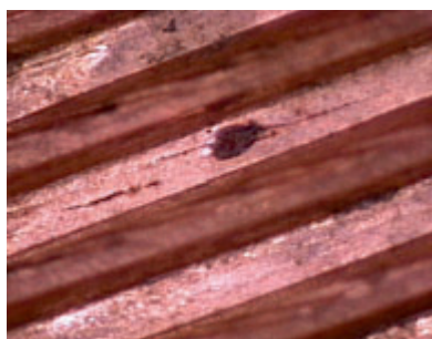
Figure 3. Corrosion Pit in Grooved Copper Tube (Photo Courtesy of Corrosion Testing Laboratories, Inc.)[1].
