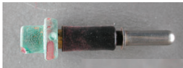
Figure 7. Dezincification of Commercial Bronze Wax Actuator from a Water Supply System (Photos Courtesy of Corrosion Testing Laboratories, Inc.)[1].
