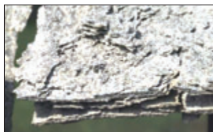
Figure 5. Exfoliation of an Aluminum Alloy in a Marine Environment[2].
