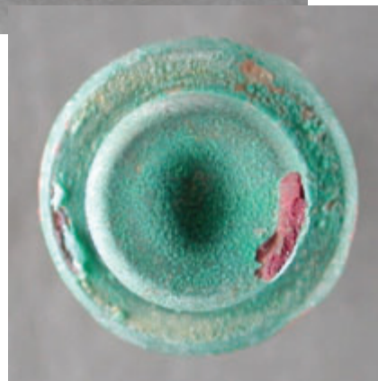
Figure 7. Dezincification of Commercial Bronze Wax Actuator from a Water Supply System (Photos Courtesy of Corrosion Testing Laboratories, Inc.)[1].
