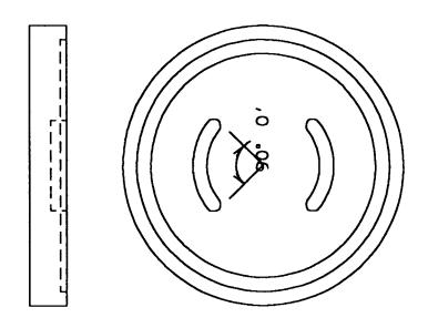
BALL BEARING / PIN STOP SLOTS
