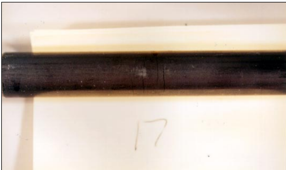
Figure 25. Specimen #17 bend test sample showing compression side (top) and tension side (bottom).
