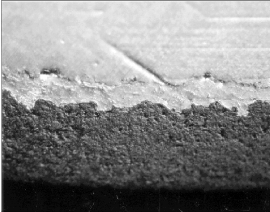
Figure 1. Cross section of alumina-13% titania coating with nickel-chrome interlayer and no seal coat (Specimen 1).
