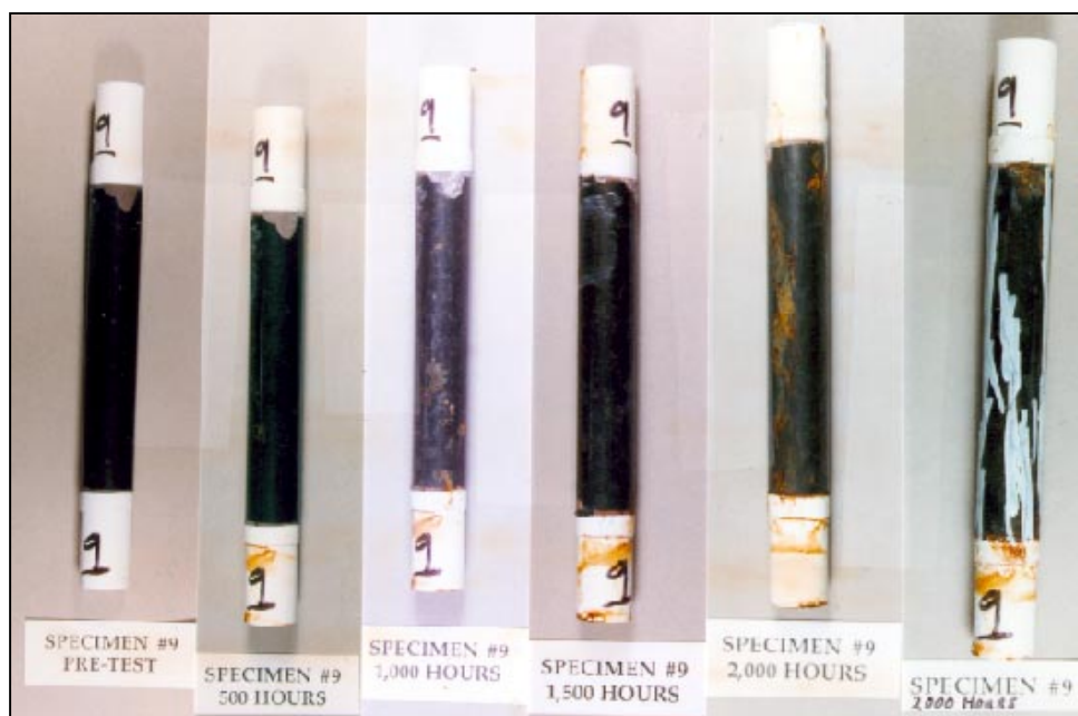
Figure 23. Specimen #9 showing the results of the salt spray test; the last frame shows the cracks outlined in white.
