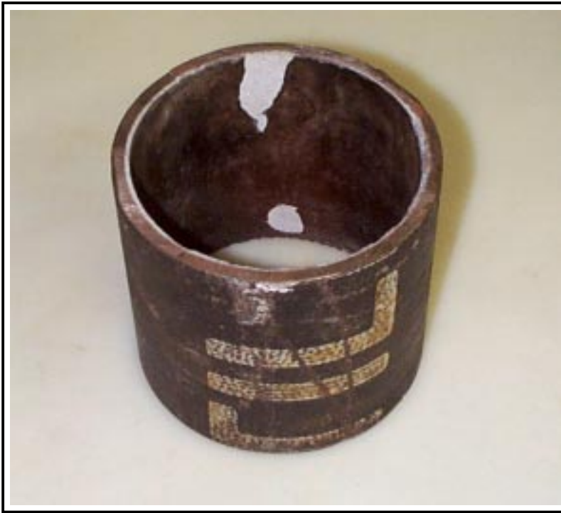
Figure 3. Inside of pipe sample where struck with sledgehammer.
