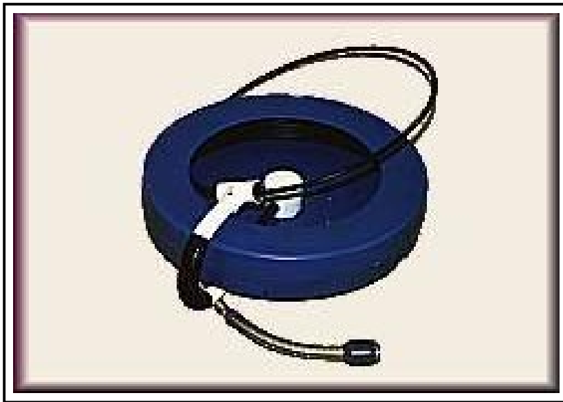
Figure 4. Scooter video camera system.
