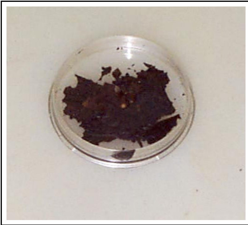
Figure 1. Uncured coating recovered following flushing.
