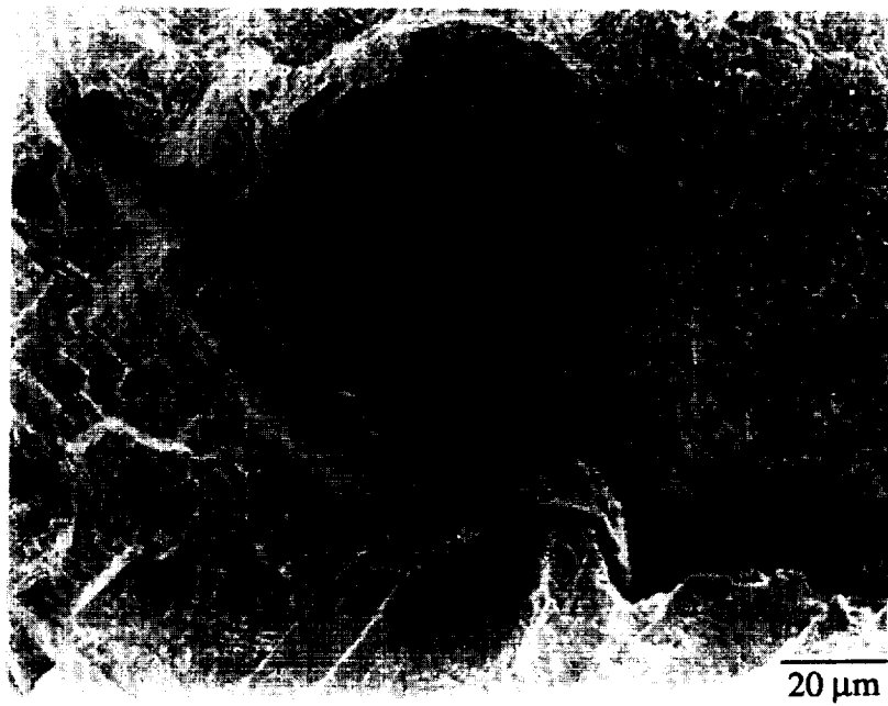
Figure 4.41 Secondary crack emanating from a pore on K_{IC} fracture surface.
