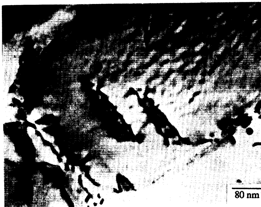
Figure 4.18 Superlattice intrinsic stacking faults occasionally observed in \gamma precipitate.
