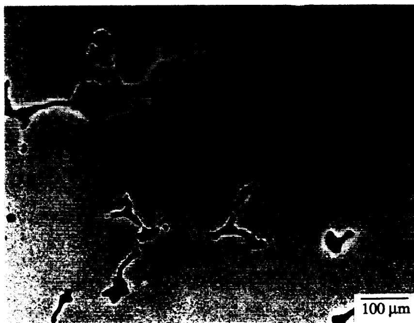
Figure 3.1 Incipient melting that infrequently occurred during heat treatment.
