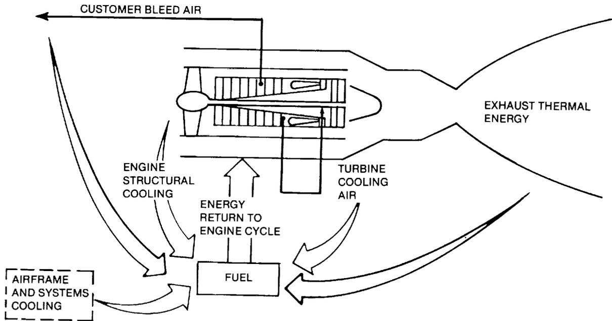
**FIGURE 2-55. WASTE HEAT RECOVERY CONCEPTS BENEFIT THE TOTAL AIRCRAFT/ENGINE**
