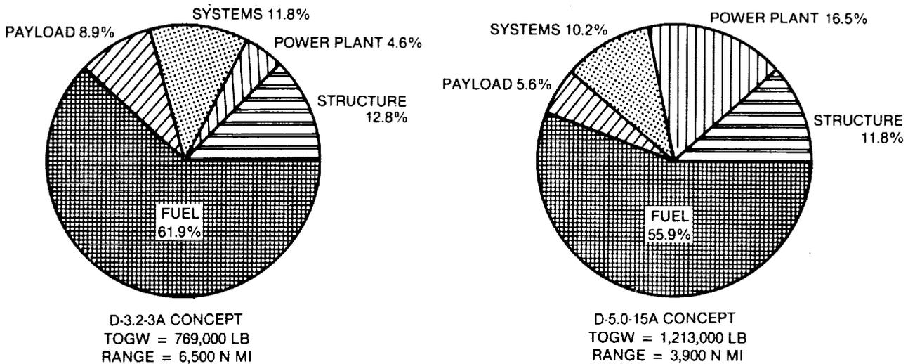
**FIGURE 2-83. HIGH-SPEED CIVIL TRANSPORT CONCEPT DESIGN WEIGHT BREAKDOWN**
