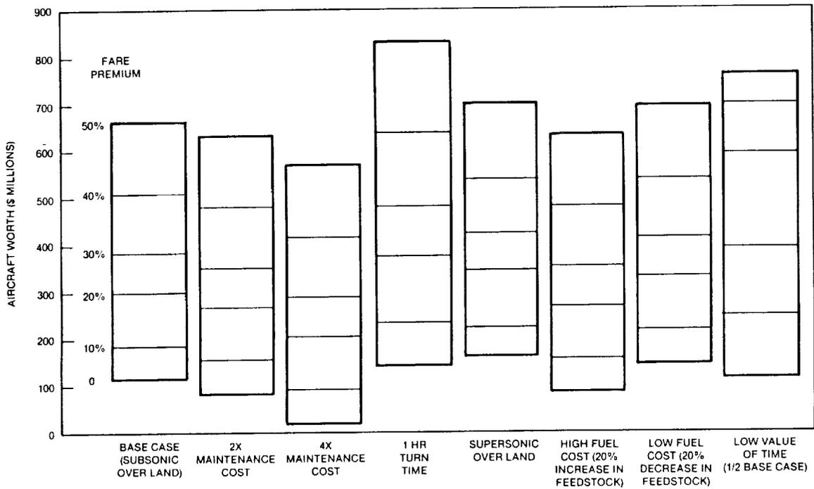
**FIGURE 3-32. SENSITIVITY OF AIRCRAFT WORTH TO ASSUMPTIONS — D3.23A
