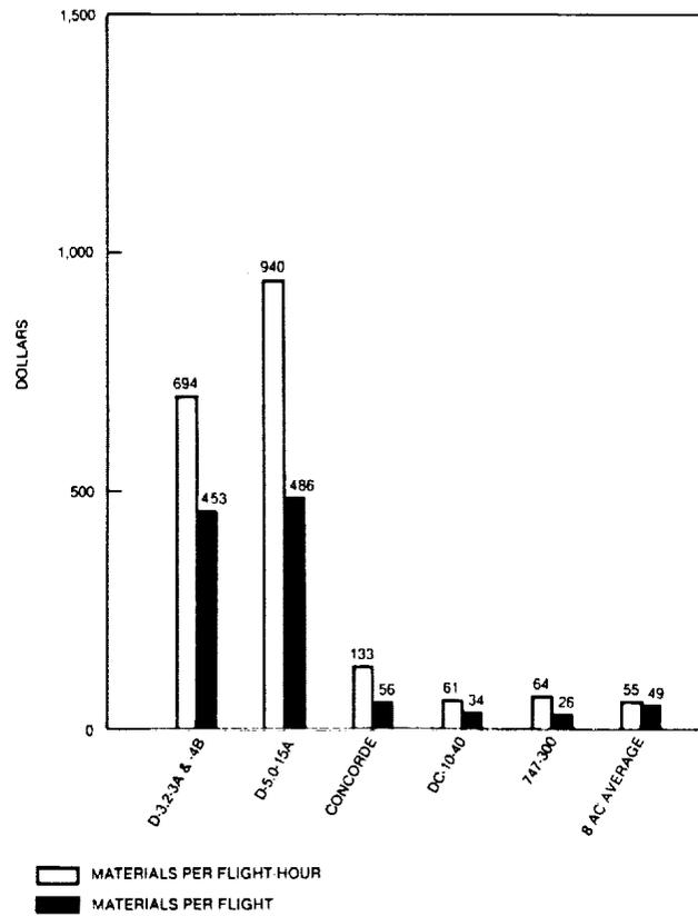
**FIGURE 3-19. ENGINE MAINTENANCE MATERIAL COSTS BASELINE VALUES**
