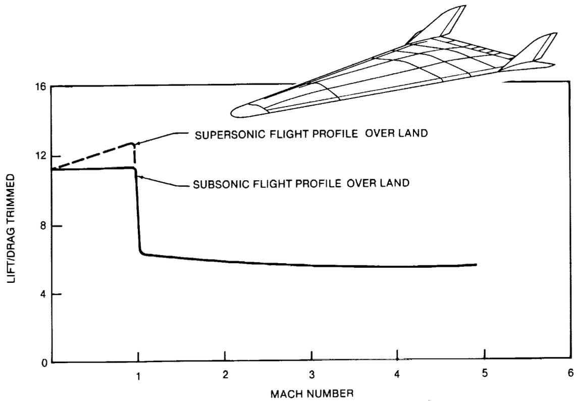
**FIGURE 2-33. LIFT/DRUM VERSUS MACH NUMBER — D5.0-15A CONCEPT**
