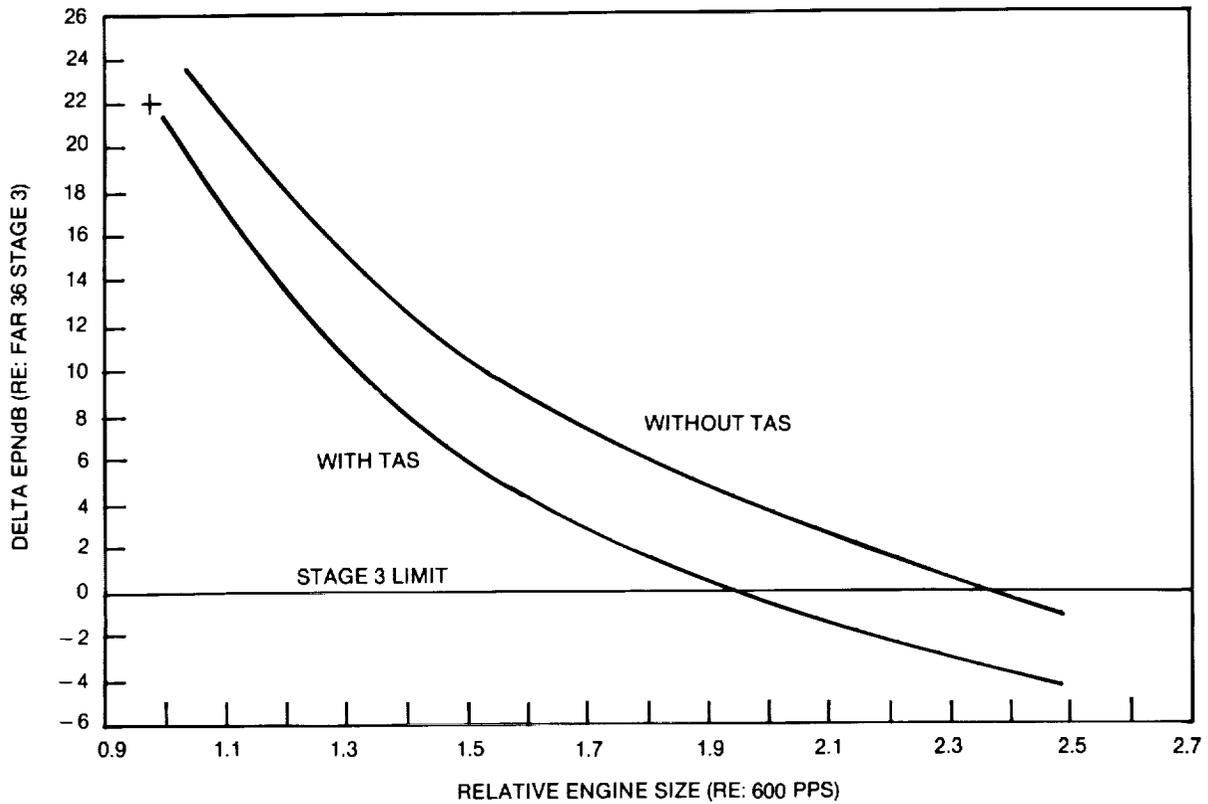
**FIGURE 4-10. P&W MACH 3.2 VSCE DATA — SIDELINES NOISE VERSUS ENGINE SIZE — SUPPRESSED CYCLE PER FNT = 57,000 LB**
