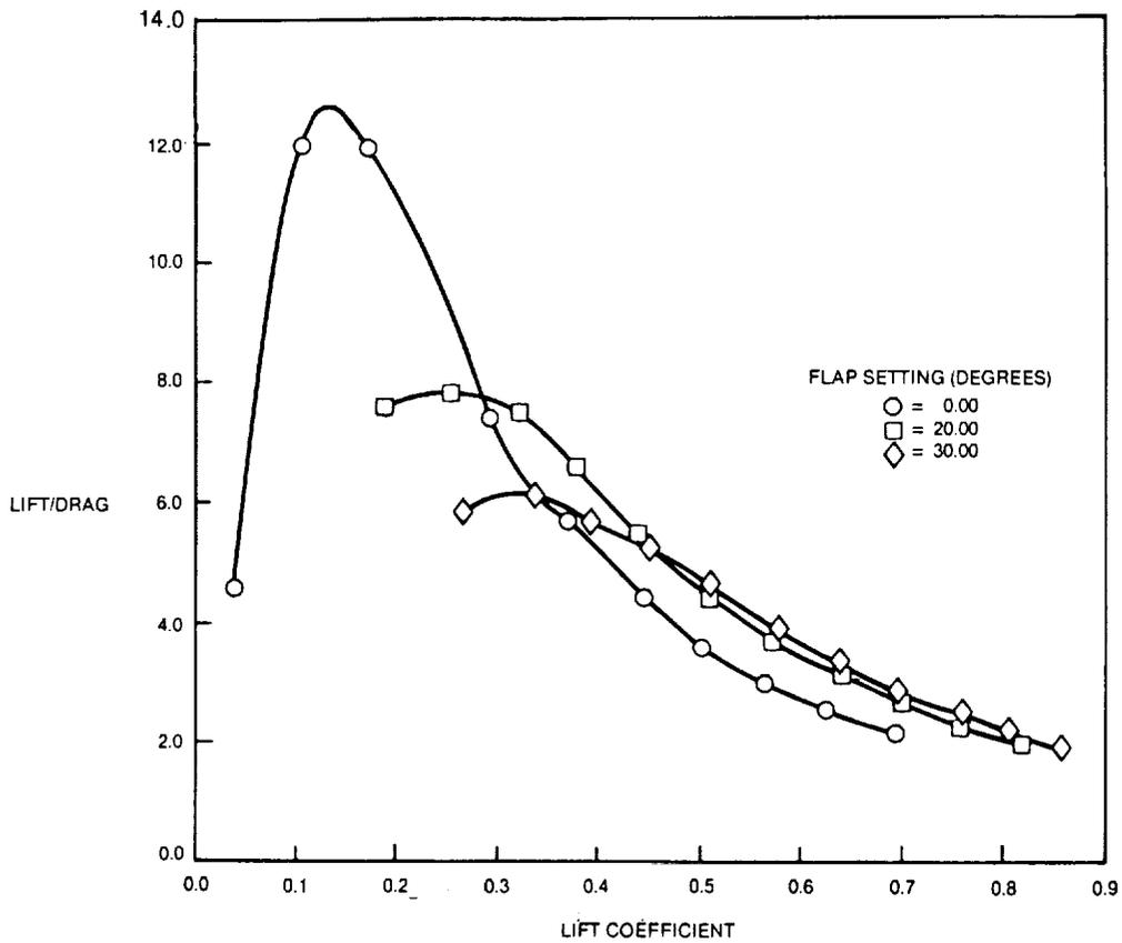
FIGURE 2-20. TRIMMED LOW-SPEED LIFT/DRAG — D3.2-3A CONCEPT LEADING EDGE SCHEDULE R
