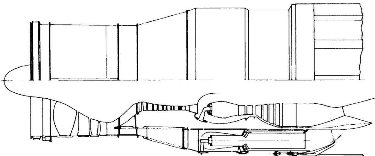
**FIGURE 2-38. P&W MACH 3.2 VSCE DUCT BURNING TURBOFAN**
