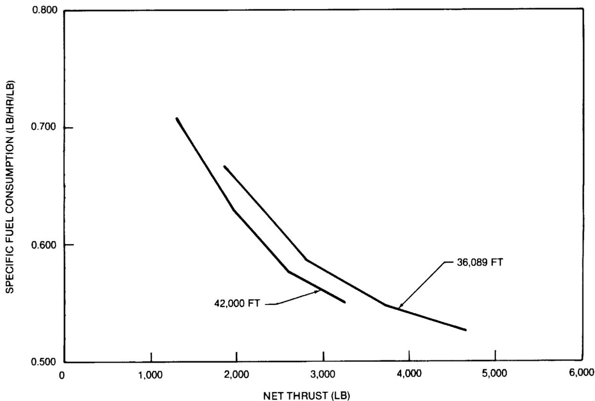
**FIGURE 2-37. P&W MACH 0.85 ADVANCED DUCTED PROP — INSTALLED CRUISE SPECIFIC FUEL CONSUMPTION**
