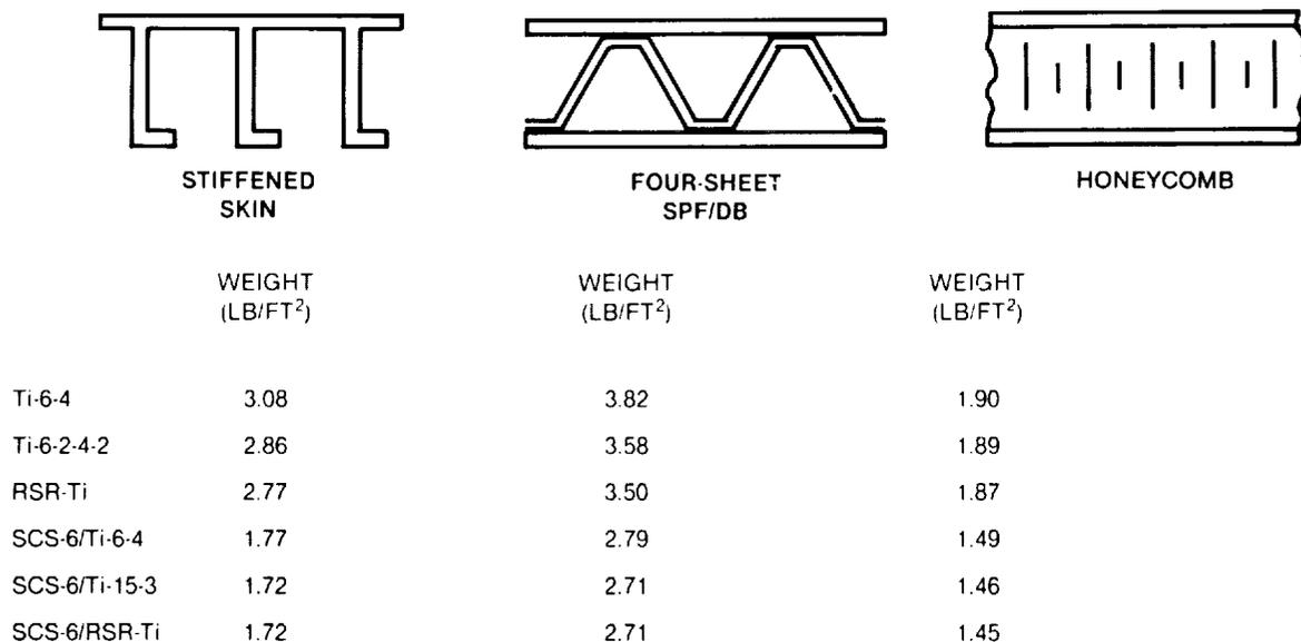
**FIGURE 2-81. STRUCTURAL PANEL WEIGHTS FOR MACH 5.0 AIRCRAFT WING**
