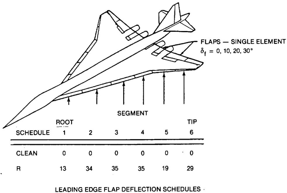
FIGURE 2-12. HIGH LIFT SYSTEM FOR D3.2-3A AND D3.2-4B CONCEPTS
