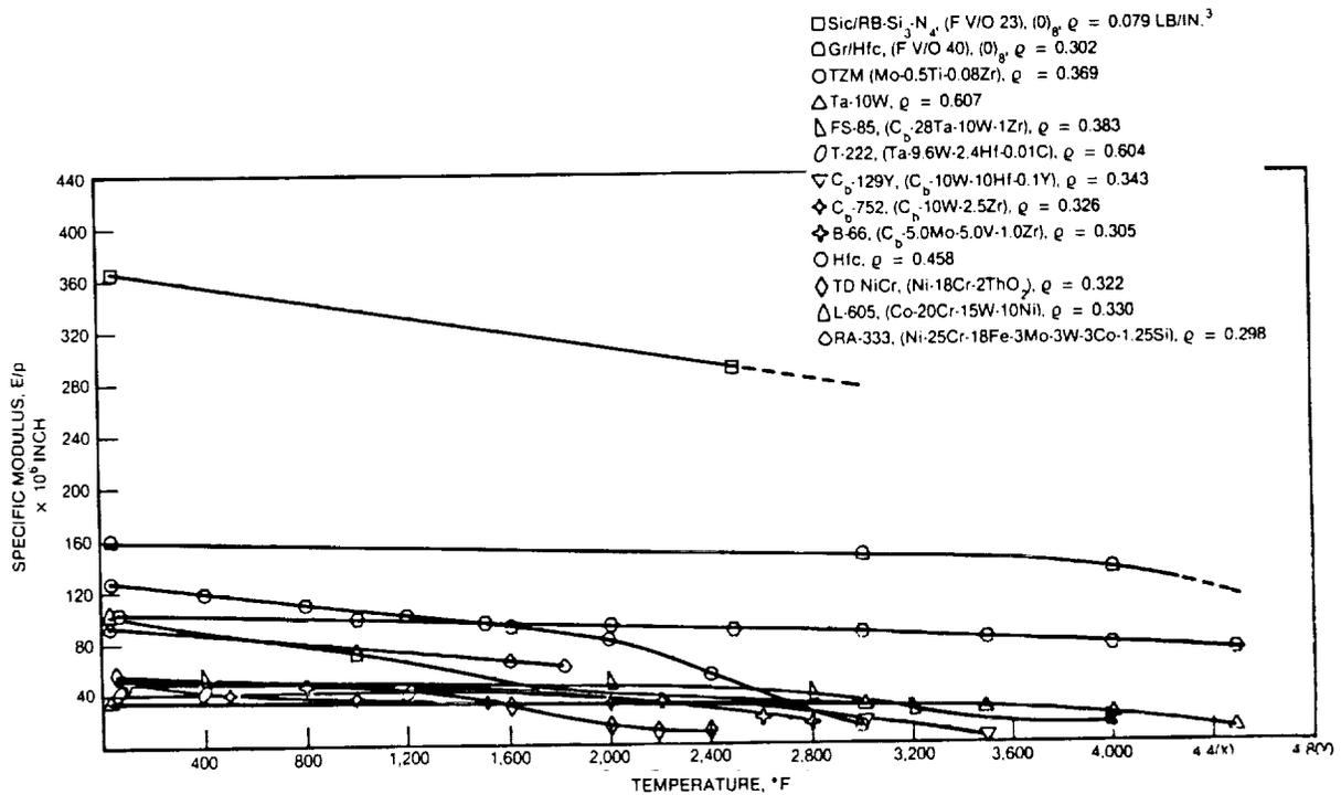
**FIGURE 2-78. SPECIFIC MODULUS OF MACH 5.0 PROPULSION SYSTEM CANDIDATE MATERIALS**
