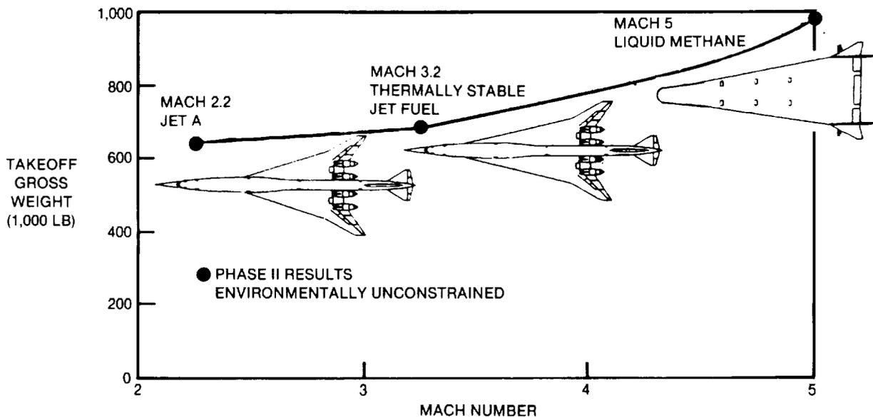
**FIGURE 1-14. PHASE II MACH NUMBER — GROSS WEIGHT 300 SEATS/6,500 NAUTICAL MILES**
