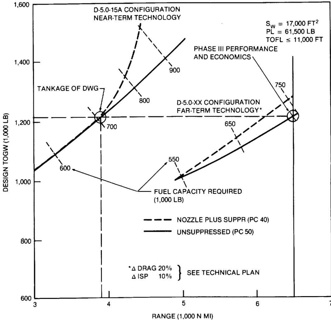
FIGURE 3-10. PHASE III MACH 5.0 SIZINGS VERSUS TECHNOLOGY AND POWER CODE
