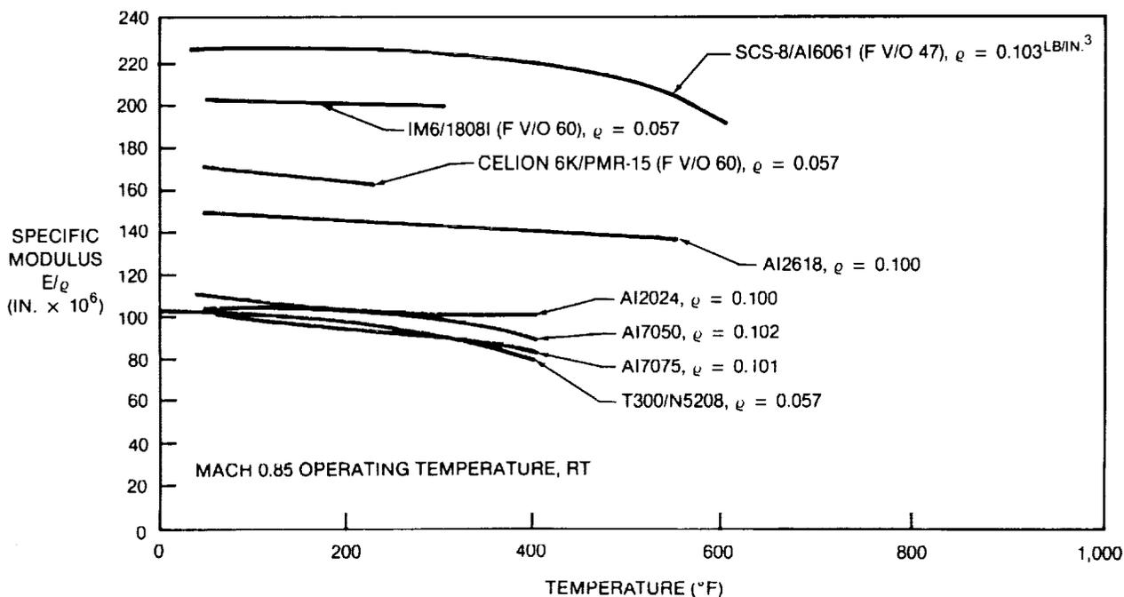
FIGURE 2-67. SPECIFIC MODULUS OF MACH 0.85 CANDIDATE MATERIALS
