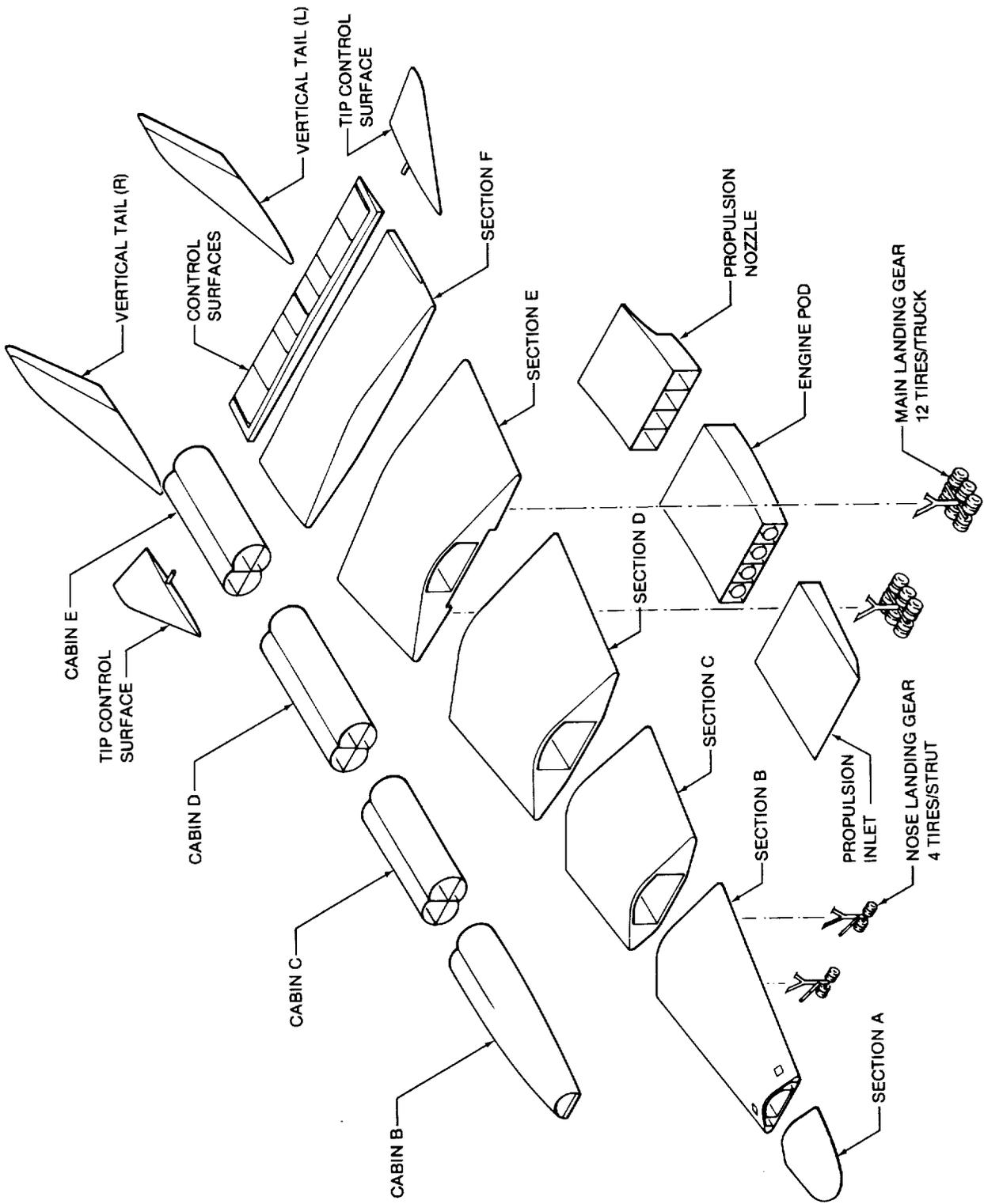
FIGURE 2-10. D5.0-15A CONCEPT PRODUCTION BREAKDOWN
