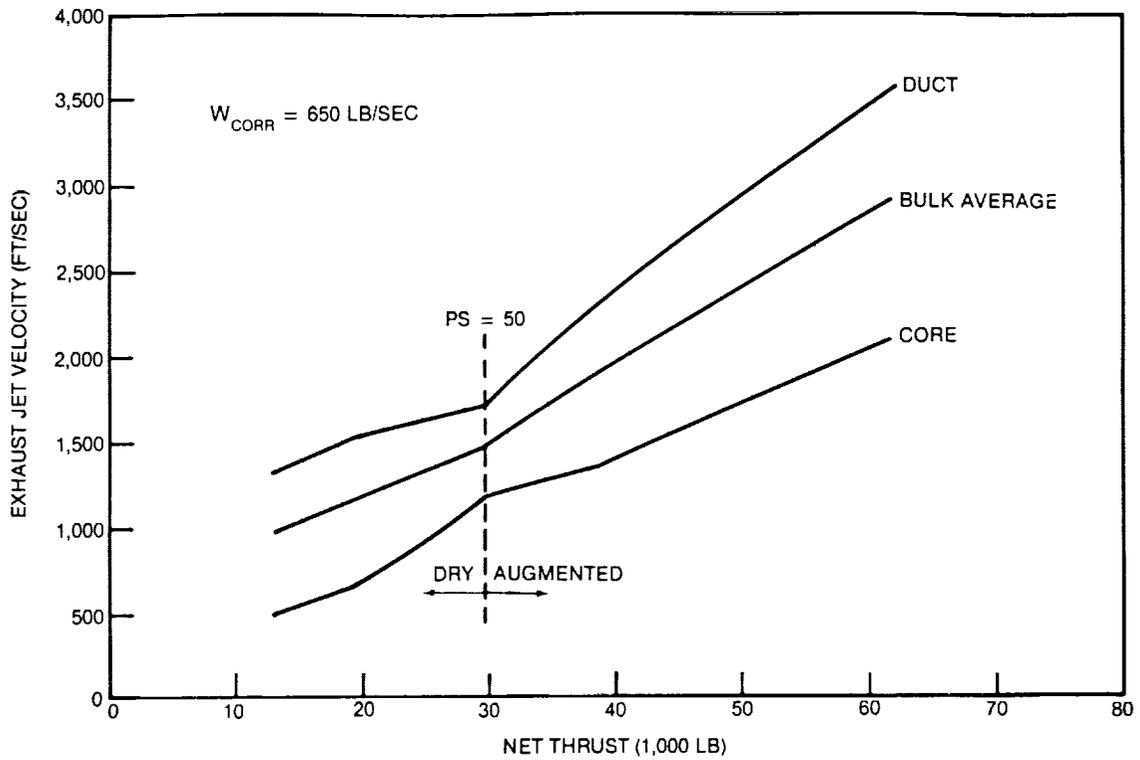
FIGURE 2-39. P&W MACH 3.2 VSCE DUCT BURNING TURBOFAN, JET VELOCITY, SEA LEVEL STATIC TAKEOFF
