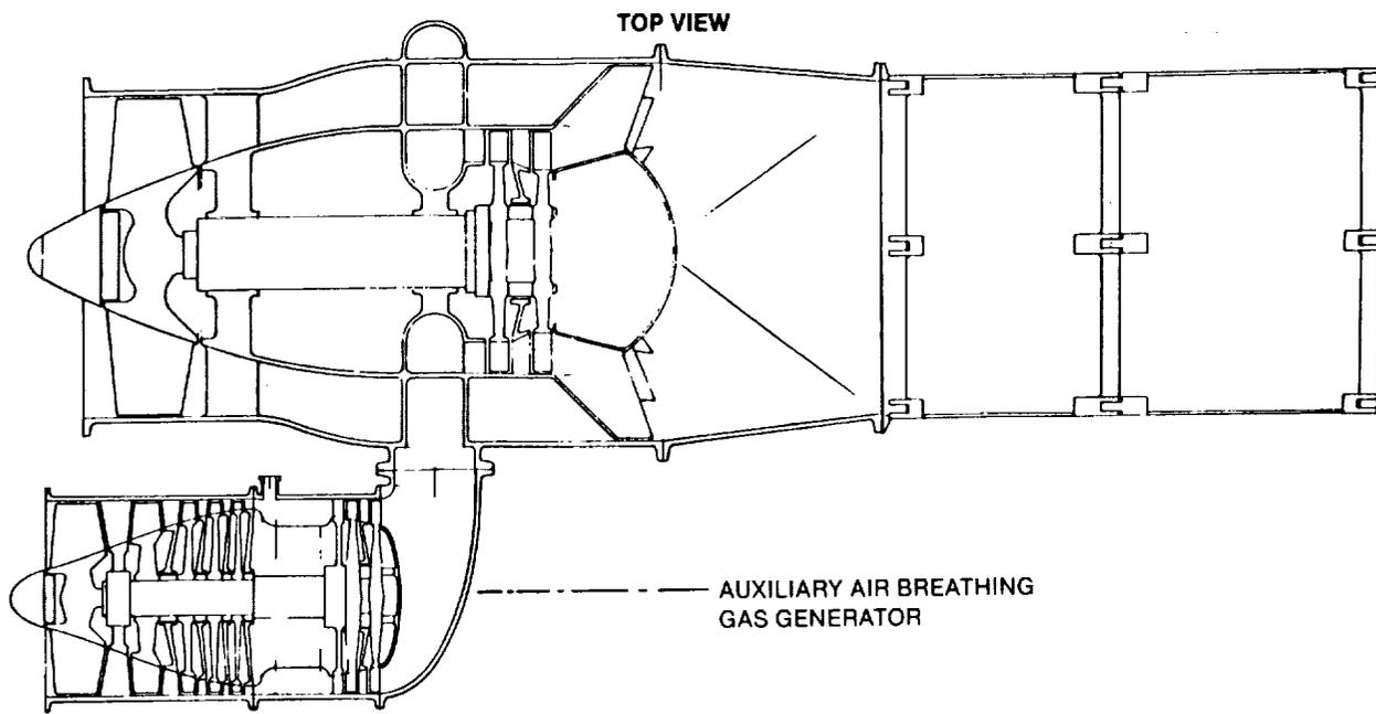
**FIGURE 2-53. AEROJET TECHSYSTEMS MACH 5.0 TWO-SPOOL ATR ENGINE**
