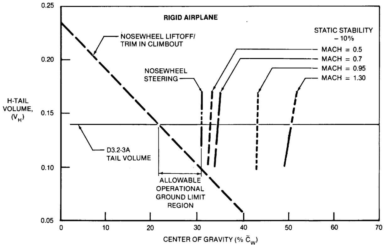
FIGURE 2-23. D3.2-3A CONCEPT ESTIMATED CENTER-OF-GRAVITY LIMITS
