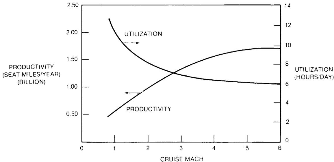
FIGURE 3-29. AIRCRAFT PRODUCTIVITY AND UTILIZATION (PHASE I DATA)
