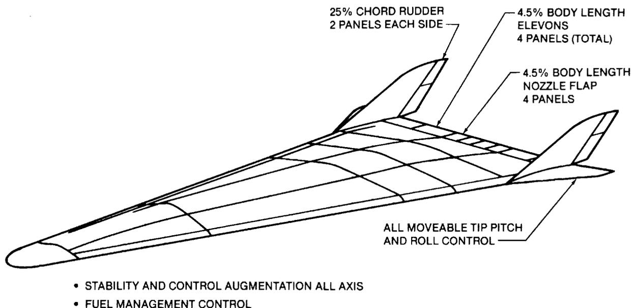
**FIGURE 2-30. D5.0-15A CONCEPT CONTROL SYSTEM DESIGN FEATURES**
