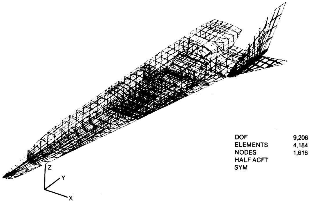
**FIGURE 2-79. FINITE ELEMENT MODEL — MACH 5.0 CONCEPT**
