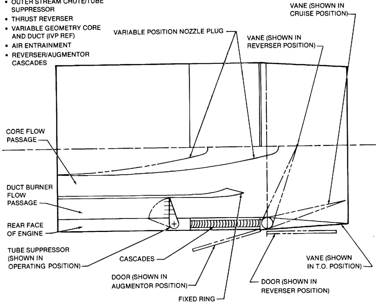
**FIGURE 2-42. MACH 3.2 NOZZLE WITH ACOUSTIC SUPPRESSION FEATURES**
