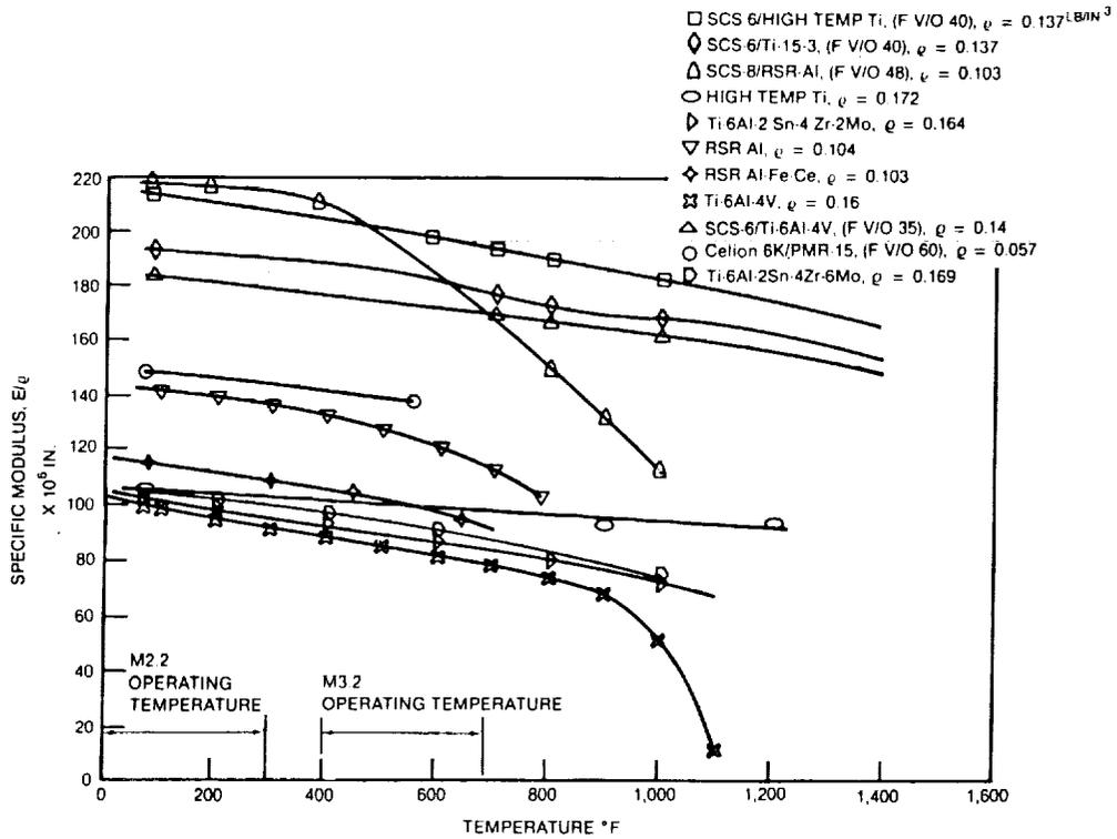
FIGURE 2-69. SPECIFIC MODULUS OF MACH 3.2 CANDIDATE MATERIALS
