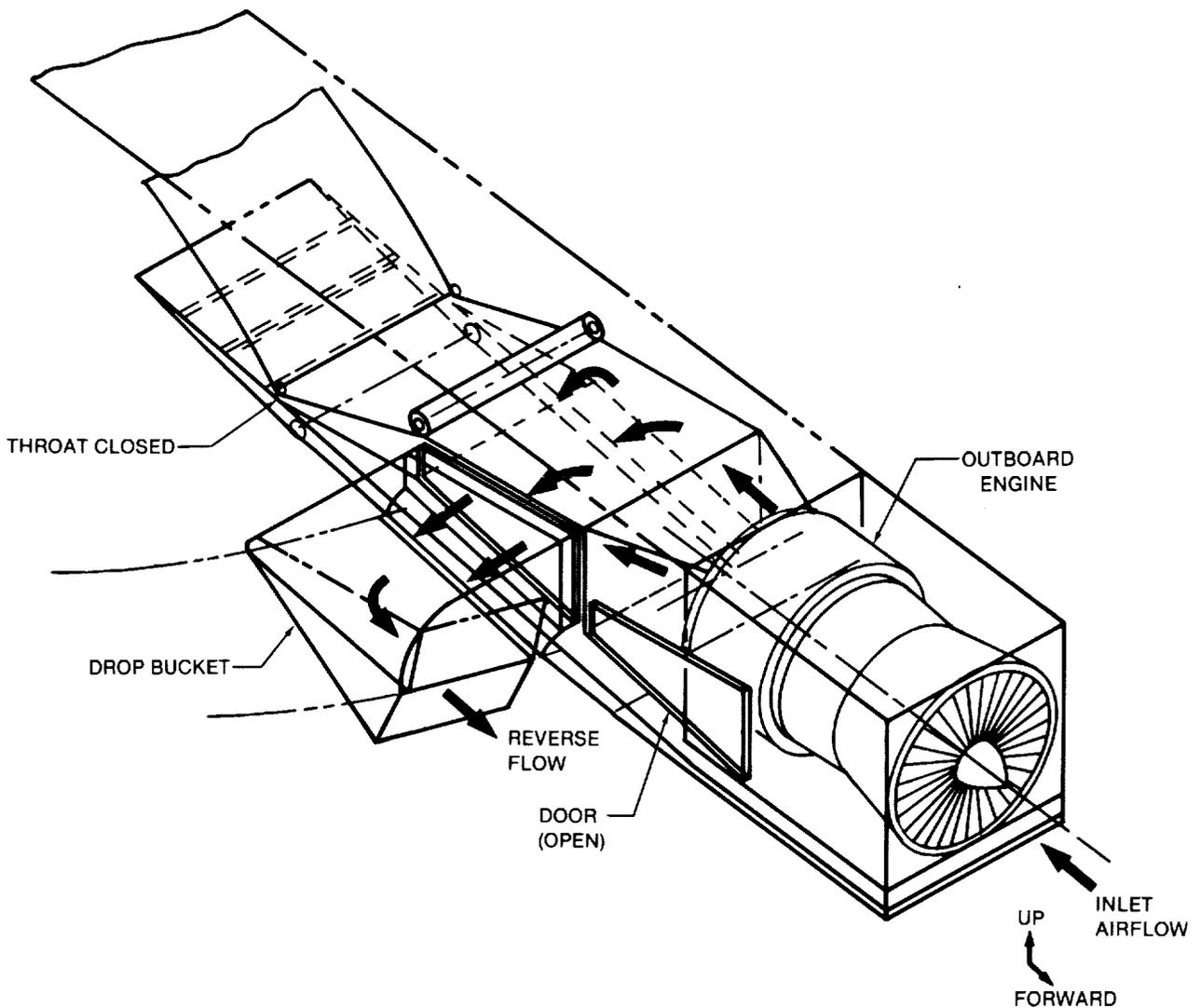
**FIGURE 2-49. MACH 5.0 THRUST REVERSER SYSTEM**
