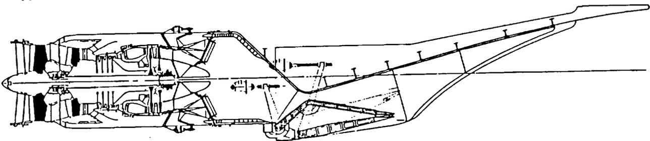
**FIGURE 2-45. MACH 5.0 SINGLE EXPANSION RAMP NOZZLE**
