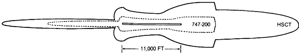
**FIGURE 4-11. 100 EPNdB NOISE CONTOURS — D3.2-3A CONCEPT**
