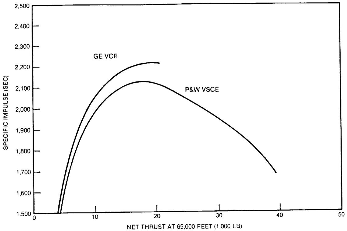
**FIGURE 2-51. COMPARISON OF INSTALLED CRUISE SPECIFIC IMPULSE FOR MACH 3.2 ENGINES**
