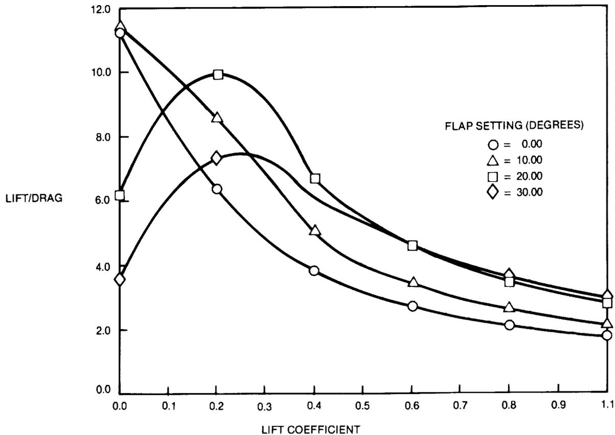
**FIGURE 2-32. TRIMMED LOW-SPEED LIFT/DRAG — D5.0-15A CONCEPT**
