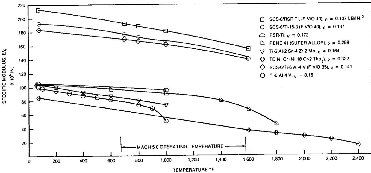
FIGURE 2-76. SPECIFIC MODULUS OF MACH 5.0 CANDIDATE MATERIALS
