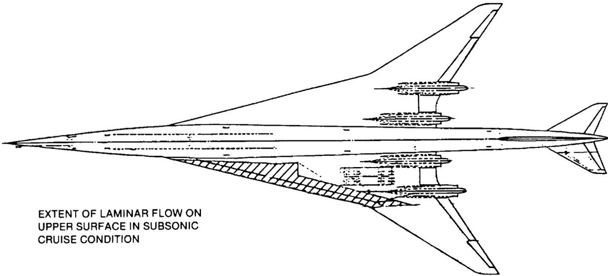
**FIGURE 2-26. EXTENT OF LAMINAR FLOW FOR D3.2-4B CONCEPT**
