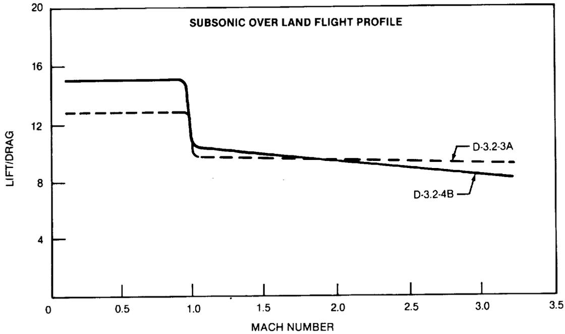
**FIGURE 2-28. LIFT/DRAGE VERSUS MACH NUMBER — D3.2-4B CONCEPT**
