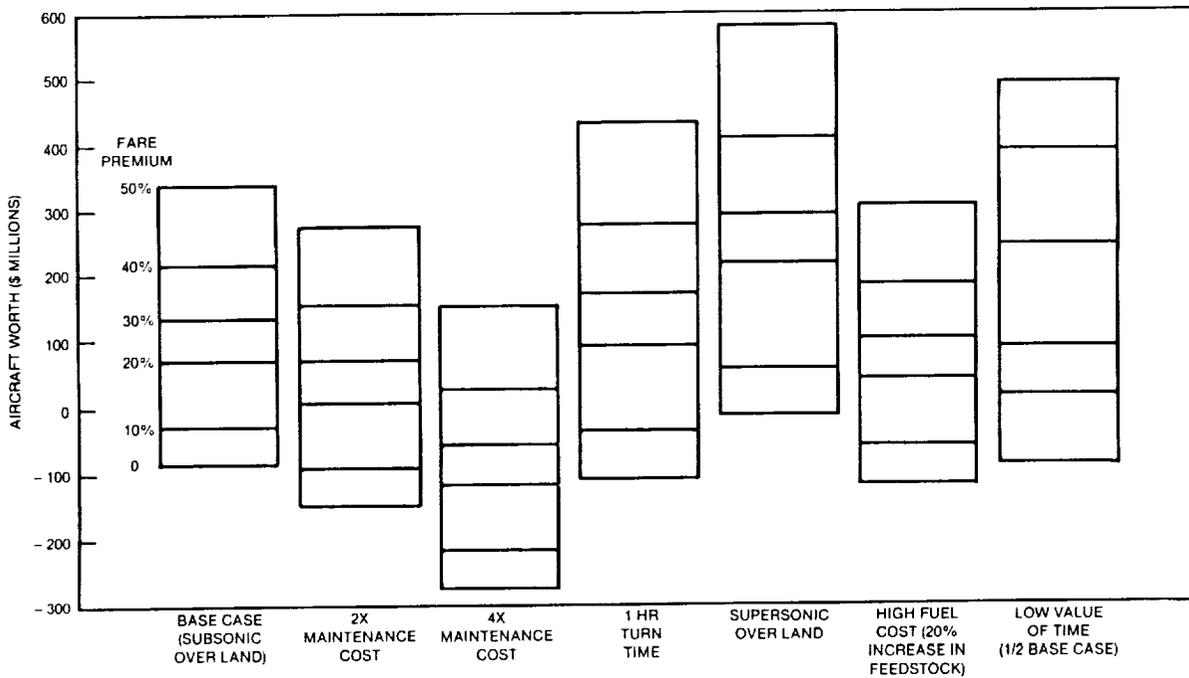
**FIGURE 3-33. SENSITIVITY OF AIRCRAFT WORTH TO ASSUMPTIONS — D5.0-15A
