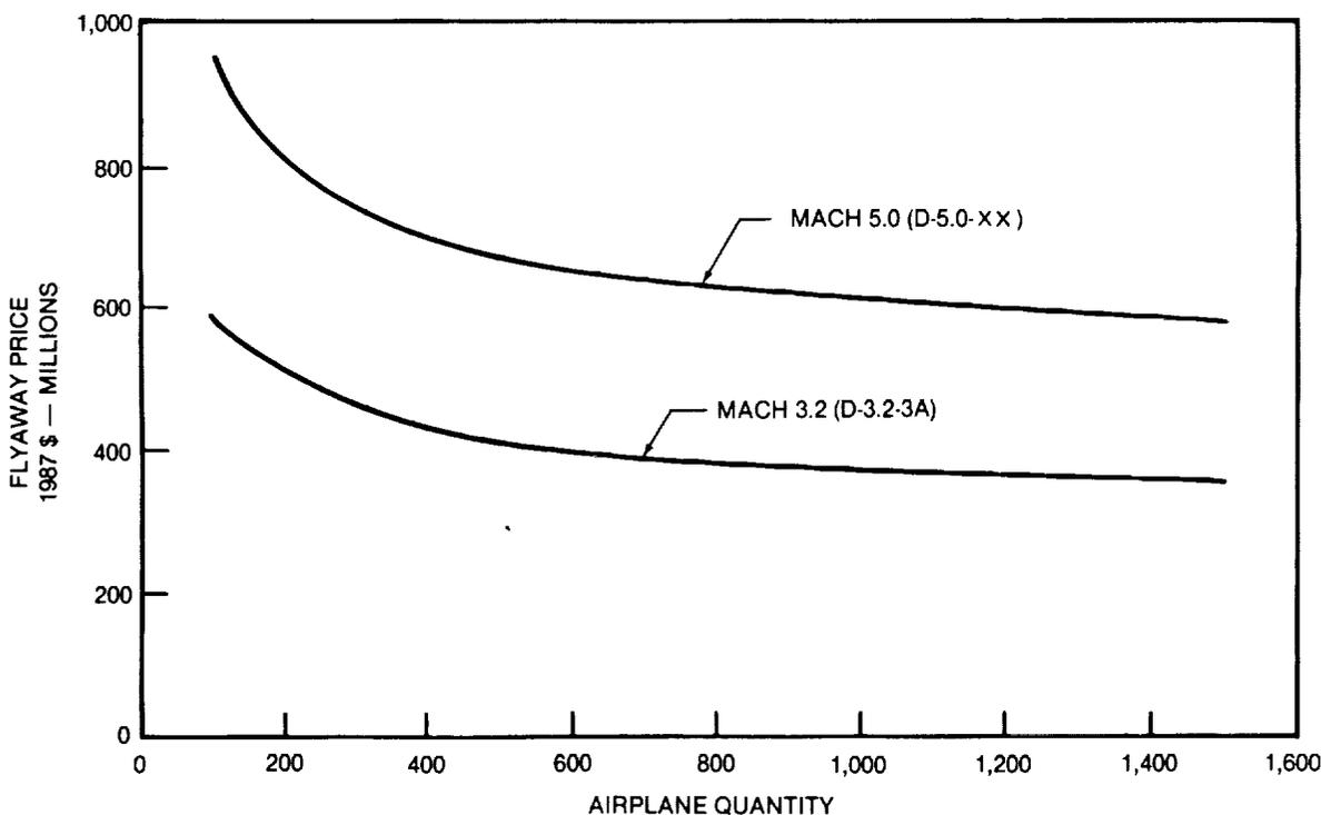
**FIGURE 3-30. CUMULATIVE AVERAGE PRICE VERSUS QUANTITY PRODUCED — MACH 3.2 AND MACH 5.0**
