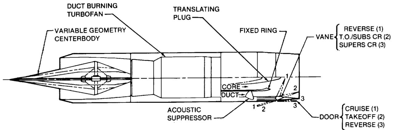
**FIGURE 2-41. MACH 3.2 NACELLE FEATURES, P&W VSCE DUCT BURNING TURBOFAN**
