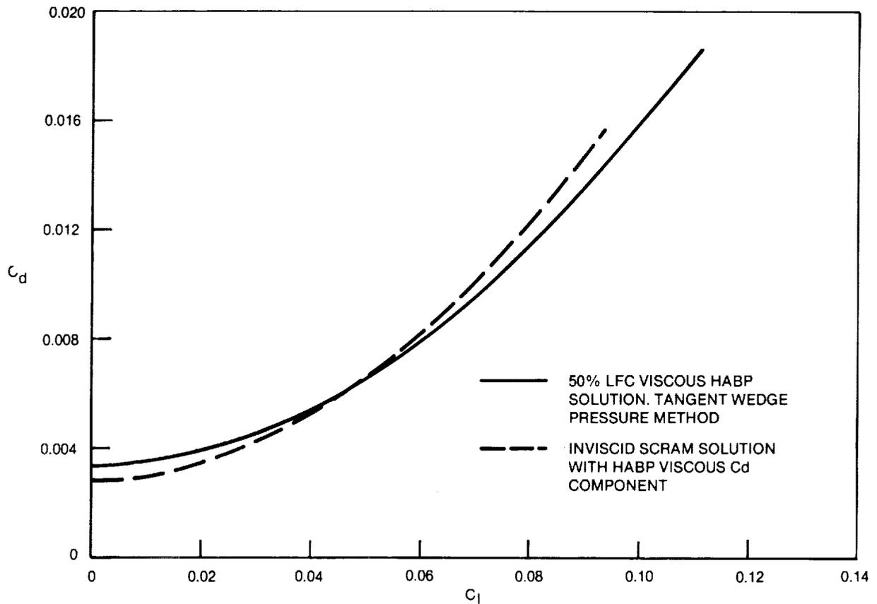
**FIGURE 2-31. HABP — SCRAM COMPARISON AT MACH 5.0, D5.0-15A CONCEPT WITHOUT VERTICAL TAIL**
