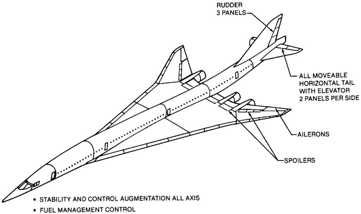
**FIGURE 2-14. D3.2-3A CONCEPT CONTROL SYSTEM DESIGN FEATURES**
