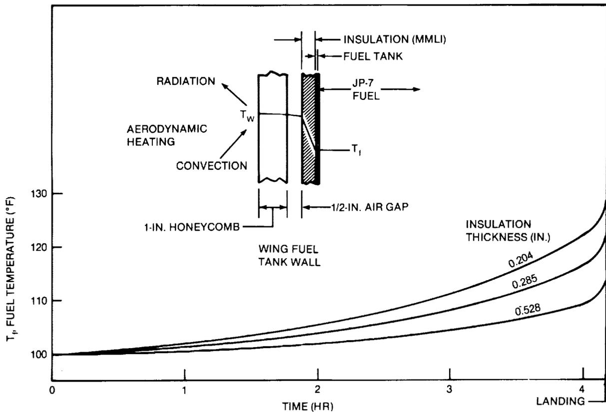
**FIGURE 2-57. MACH 3.2 VEHICLE FUEL TEMPERATURES, MMLI TANK INSULATION**
