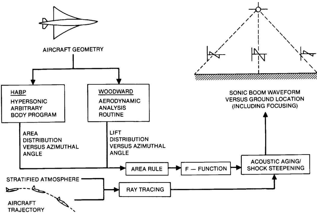
**FIGURE 4-2. SUPERSONIC BOOM PREDICTION METHODOLOGY VIA MDBOOM**
