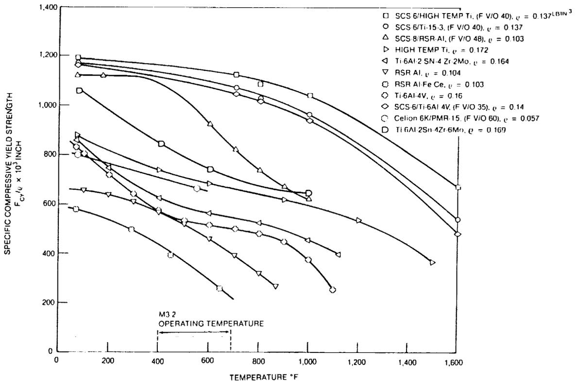
FIGURE 2-70. SPECIFIC COMPRESSIVE YIELD STRENGTH OF MACH 3.2 MATERIALS
