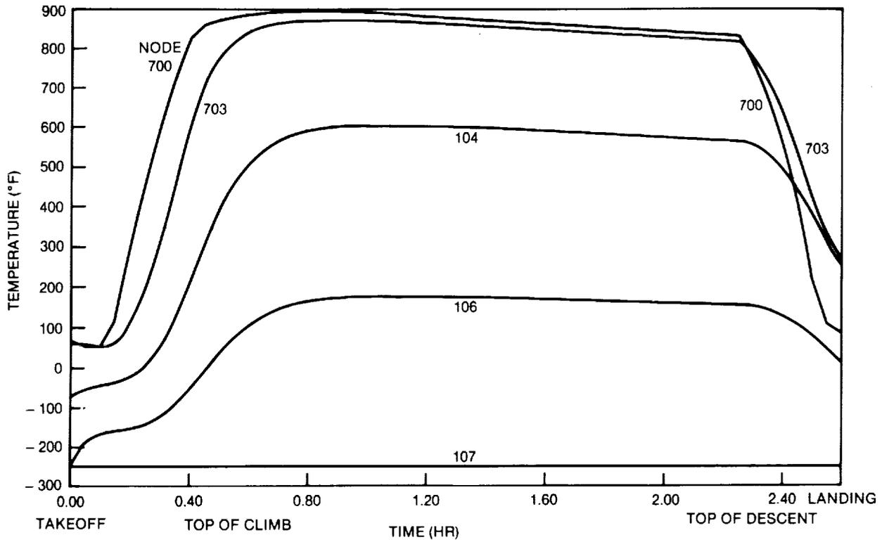
A. WING LOWER TANK SURFACE TEMPERATURES AT X = 42 FT
