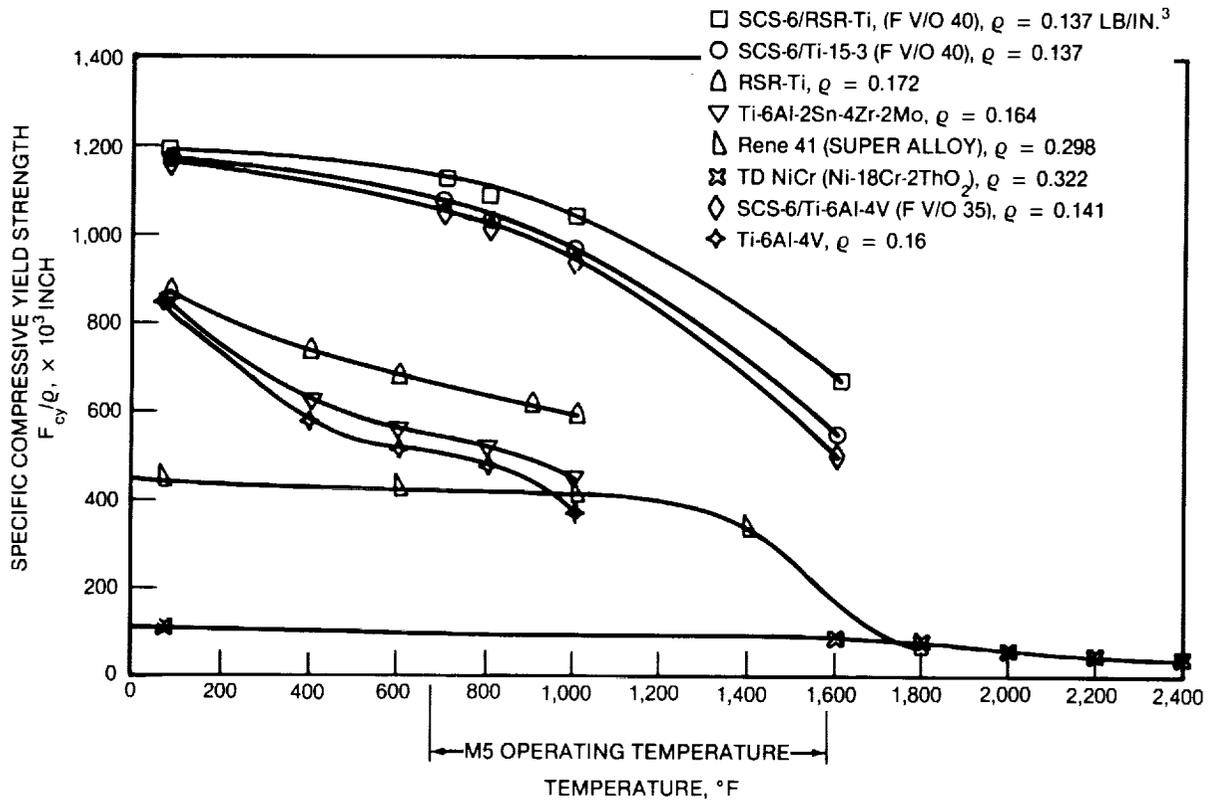
**FIGURE 2-77. SPECIFIC COMPRESSION YIELD STRENGTH OF MACH 5.0 CANDIDATE MATERIALS**
