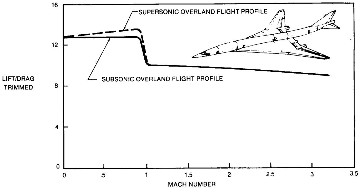
FIGURE 2-21. LIFT/DRAG VERSUS MACH NUMBER — D3.2-3A CONCEPT
