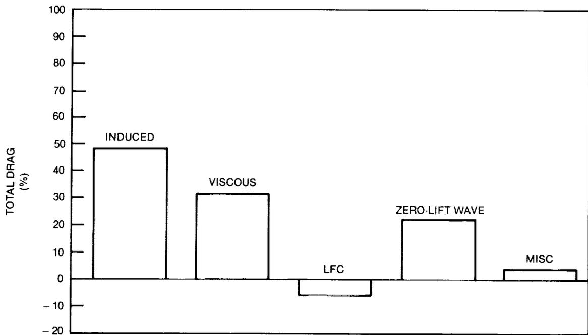
**FIGURE 2-22. DRAG BREAKDOWN — D3.2-3A CONCEPT**
