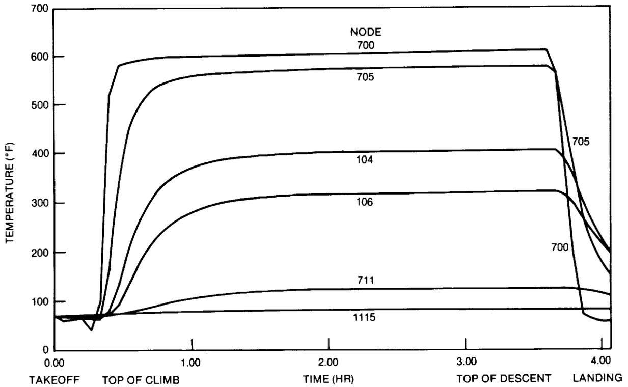
A. FUSELAGE LOWER SURFACE TEMPERATURES AT X = 20 FT
