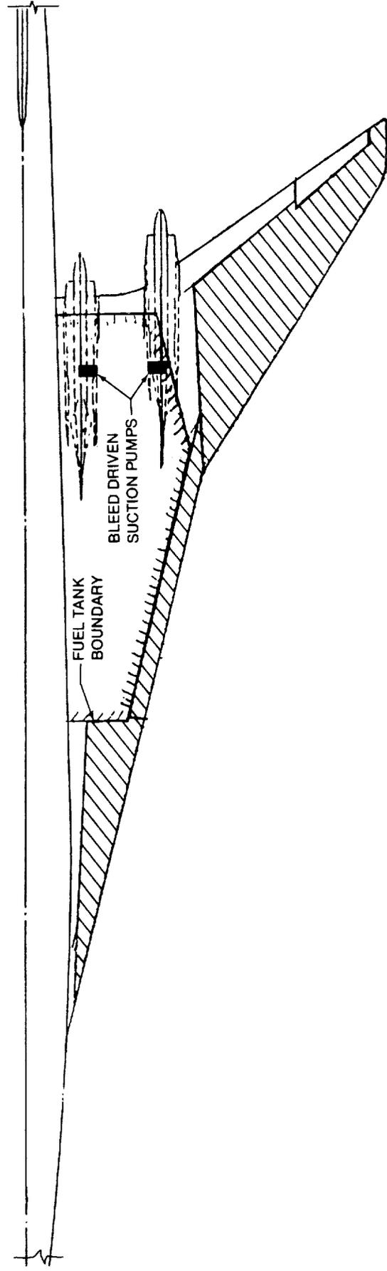
**FIGURE 2-25. LAMINAR FLOW CONTROL SUCTION REGION FOR D3.2-4B CONCEPT**
