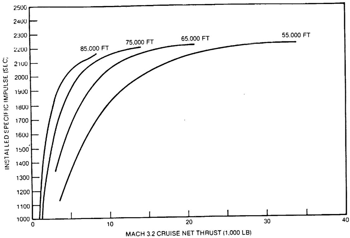
**FIGURE 2-52. GE MACH 3.2, VCE — INSTALLED CRUISE SPECIFIC IMPULSE**
