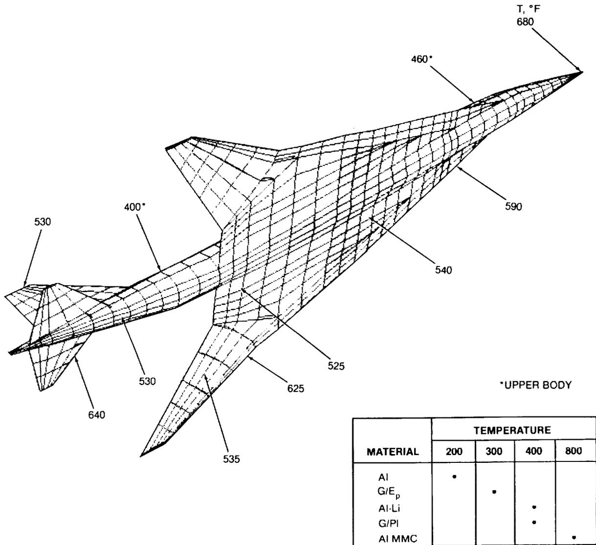
**FIGURE 2-68. MAXIMUM TEMPERATURES — CANDIDATE MATERIALS — MACH 3.2**
