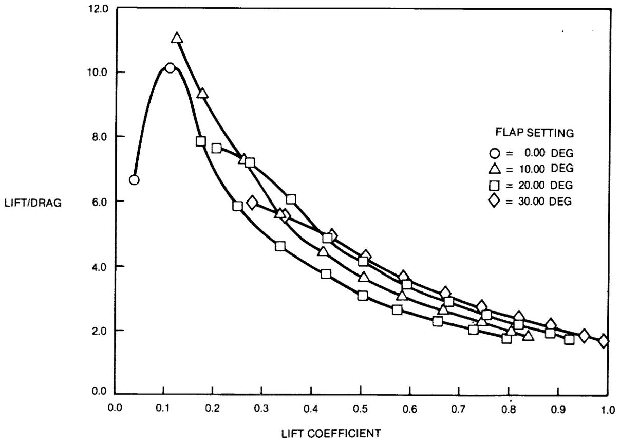
FIGURE 2-19. TRIMMED LOW-SPEED LIFT/DRAGE — D3.2-3A CONCEPT CLEAN LEADING EDGE
