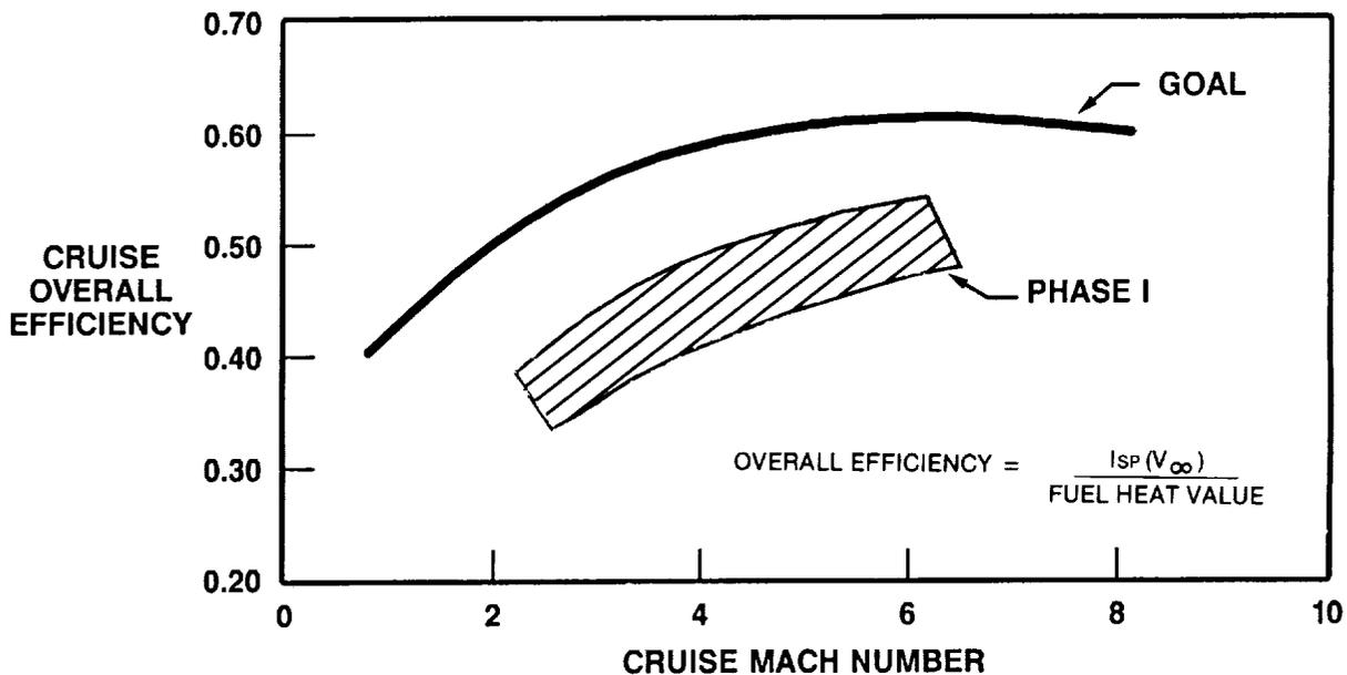
FIGURE 1-8. PROPULSION TECHNOLOGY, PHASE I
