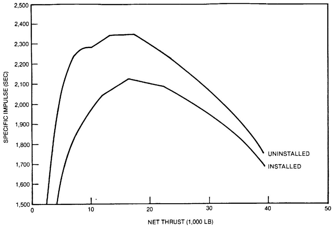
FIGURE 2-40. P&W MACH 3.2 VSCE DUCT BURNING TURBOFAN, MACH 3.2 CRUISE SPECIFIC IMPULSE AT 65,000 FEET
