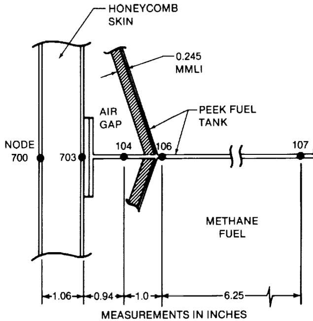
B. THERMAL MODEL FOR LOWER FUEL TANK AT X = 42 FT
