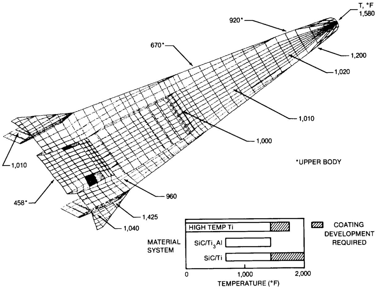
FIGURE 2-75. MAXIMUM TEMPERATURES — CANDIDATE MATERIALS — MACH 5.0 CONCEPT
