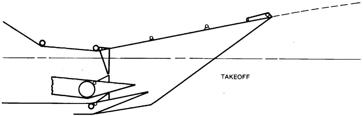
**FIGURE 2-46. GE MACH 5.0 WEDGE SUPPRESSOR NOZZLE CONCEPT**
