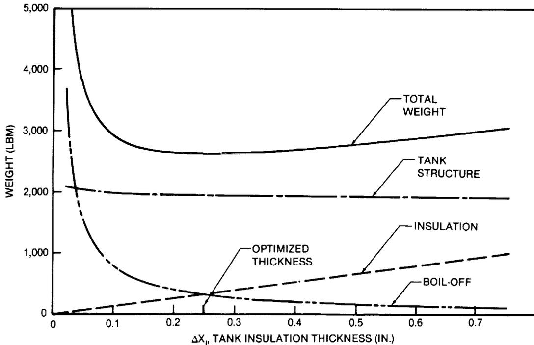
**FIGURE 2-61. FUEL TANK INSULATION OPTIMIZATION, MMLI — TANK NO. 2, LOWER SURFACE, D5.0-15A CONCEPT**
