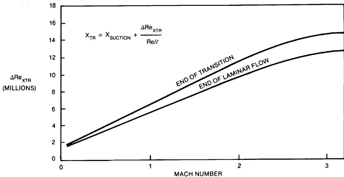
**FIGURE 2-17. TRANSITION REYNOLDS NUMBER INCREMENT (FLAT ROOFTOP)**
