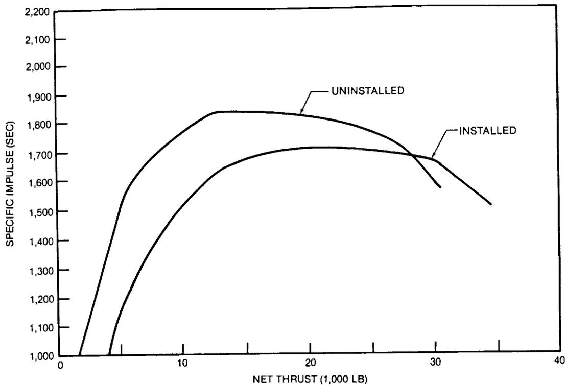
**FIGURE 2-48. GE MACH 5.0 VCHJ — INSTALLED  $I_{sp}$  AT 80,000 FEET**
