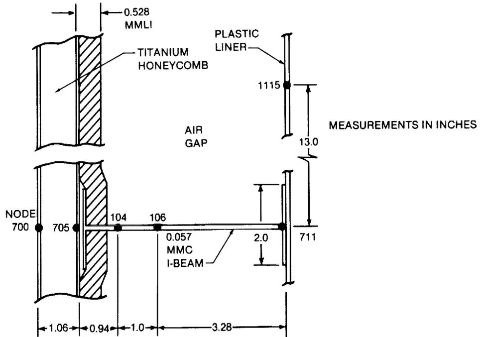
B. THERMAL MODEL FOR LOWER FUSELAGE AT X = 20 FT
