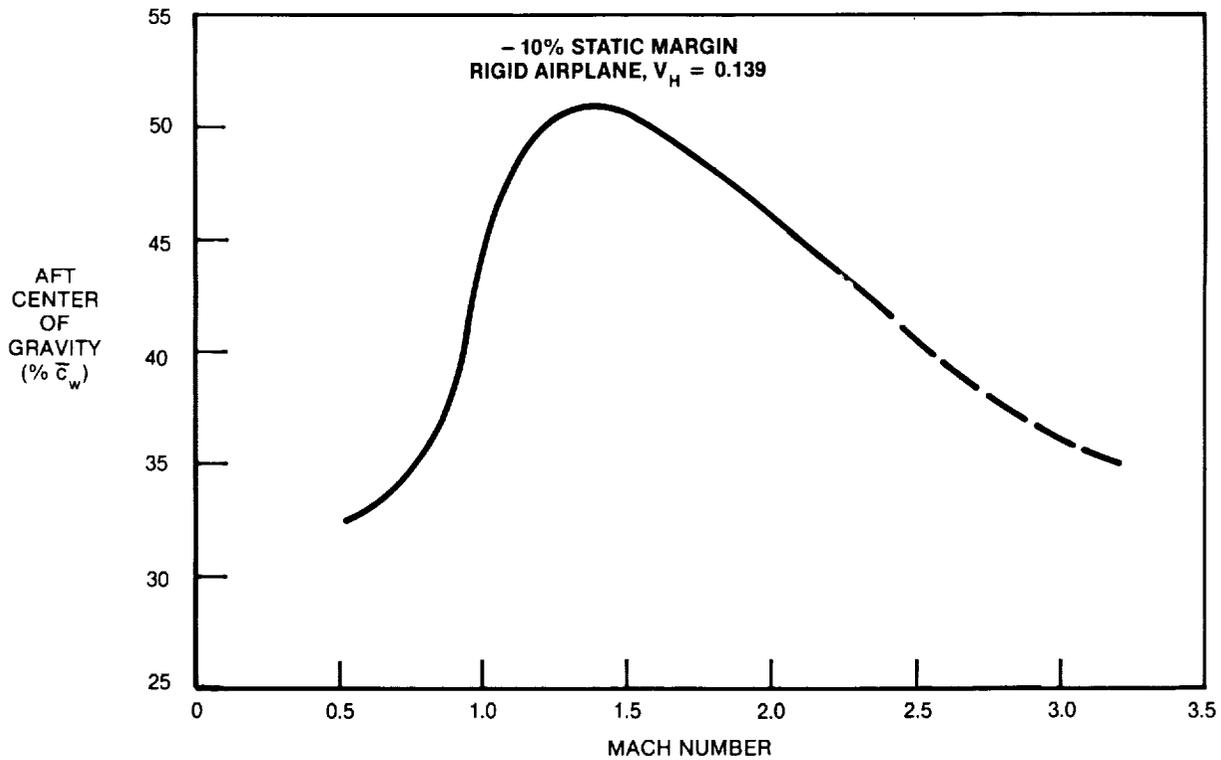
FIGURE 2-24. D3.2-3A CONCEPT ESTIMATED AFT CENTER-OF-GRAVITY LIMITS
