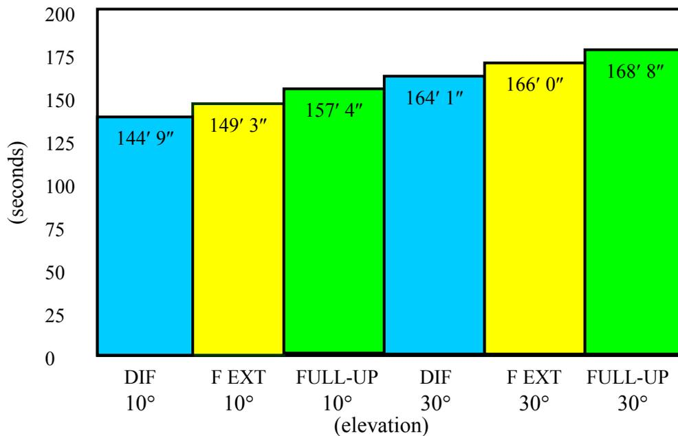
FIGURE 22. COMPARISON OF THE HIGH-PERFORMANCE, MULTIPOSITION, BUMPER-MOUNTED TURRET AGENT STREAM THROW RANGE TEST RESULTS WITH THE P-19 ROOF-MOUNTED TURRET SET AT VARIOUS POSITIONS AND DEGREES OF ELEVATION
