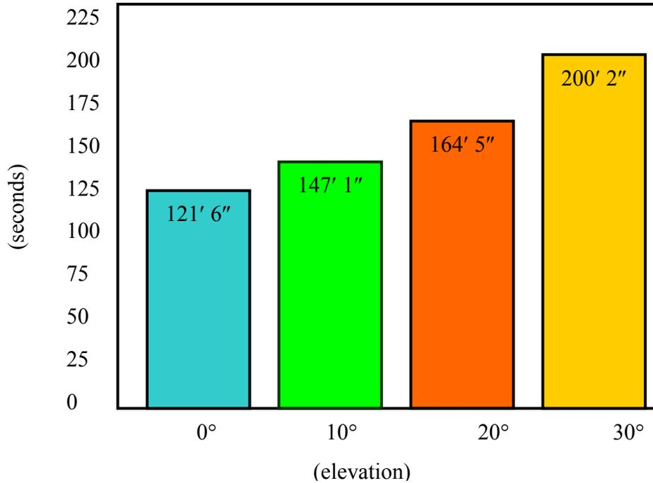
FIGURE 19c. THE HIGH-PERFORMANCE, MULTIPOSITION, BUMPER-MOUNTED TURRET WATER STREAM THROW RANGE TESTS, SET TO FULL-UP POSITION AT VARIOUS DEGREES OF ELEVATION
