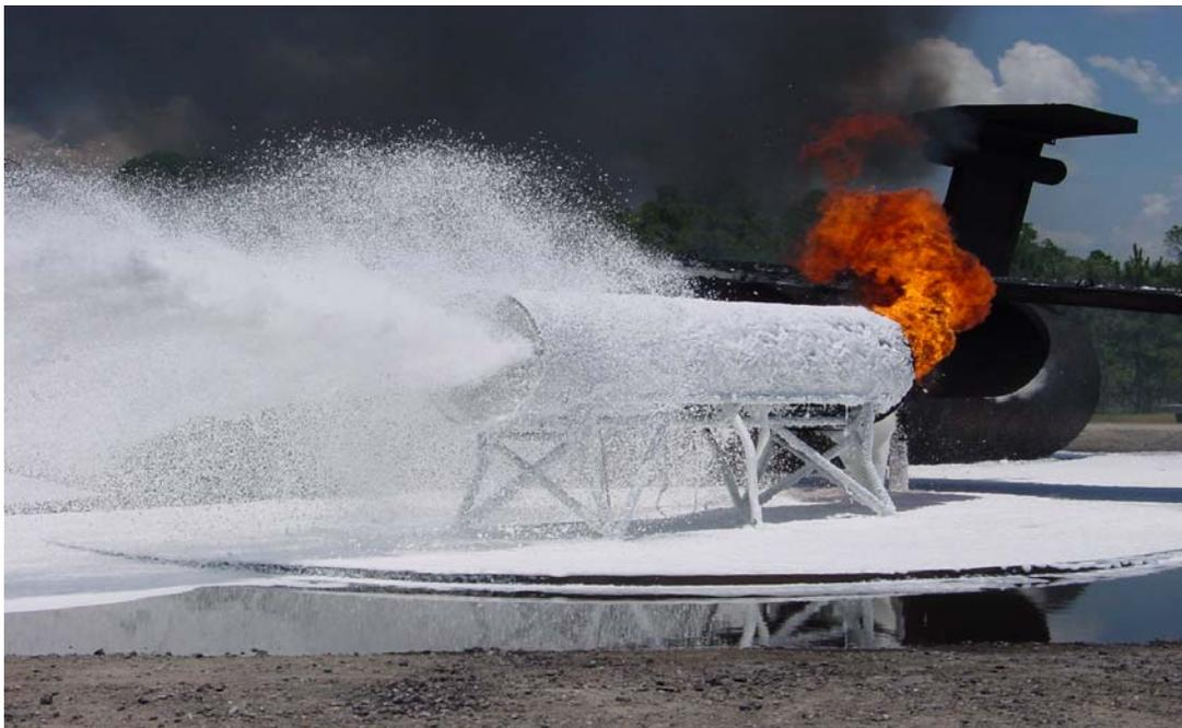
FIGURE 5. F-100 ENGINE NACELLE AND 30-ft-DIAMETER RING TEST DEVICE
