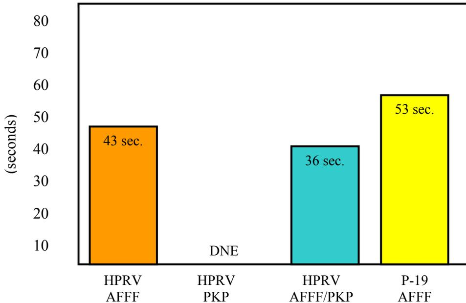
FIGURE 14. AVERAGE RESULTS OF THE TAIL-MOUNTED, HIGH ENGINE NACELLE FIRE TESTS
