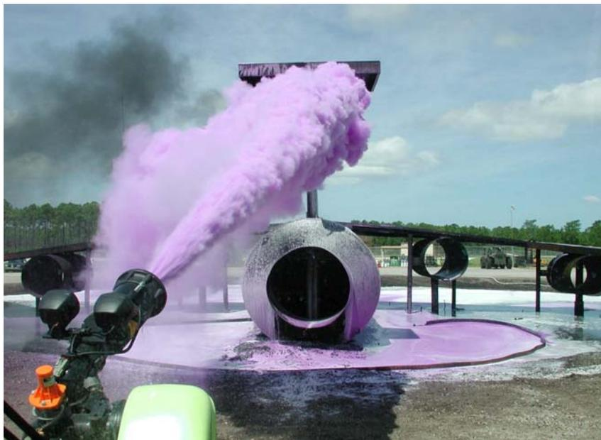
FIGURE 16. THE HIGH-PERFORMANCE, MULTIPOSITION, BUMPER-MOUNTED TURRET USING BOTH AFFF AND PKP ON A 3-D FLOWING FUEL FIRE
