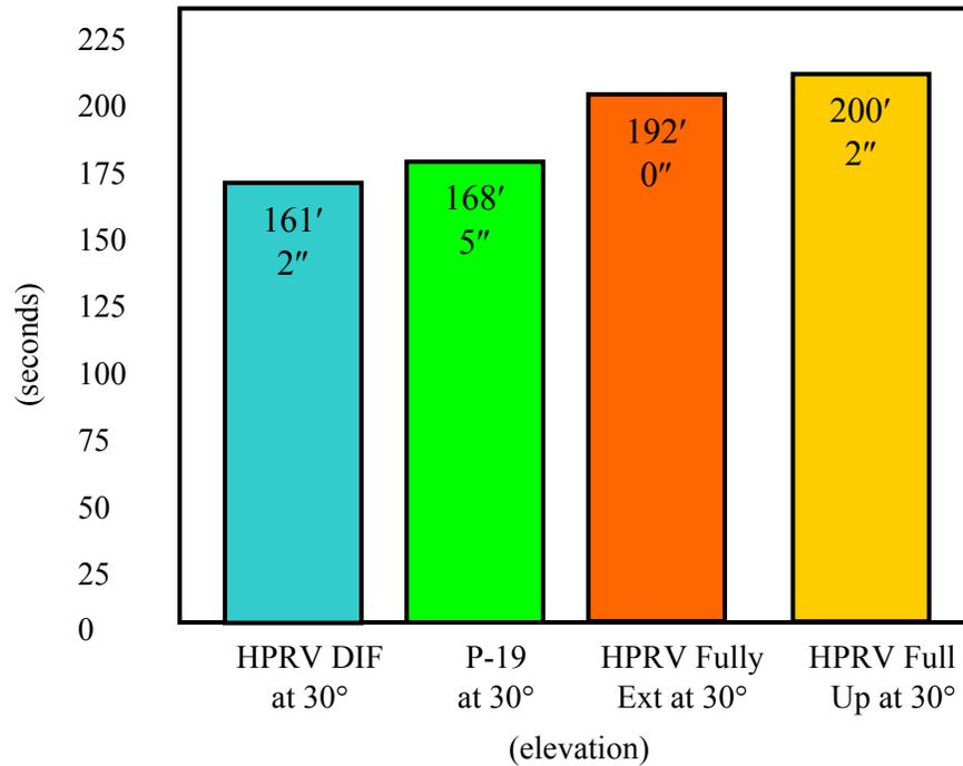
FIGURE 21. COMPARISON OF THE HIGH-PERFORMANCE, MULTIPOSITION, BUMPER-MOUNTED TURRET AND THE P-19 ROOF-MOUNTED TURRET WATER STREAM THROW RANGE TESTS AT A 30° ELEVATION
