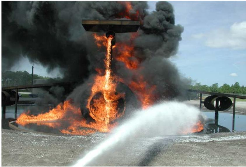
FIGURE 15. THE HIGH-PERFORMANCE, MULTIPOSITION, BUMPER-MOUNTED TURRET USING AFFF ON A 2-D POOL FIRE
