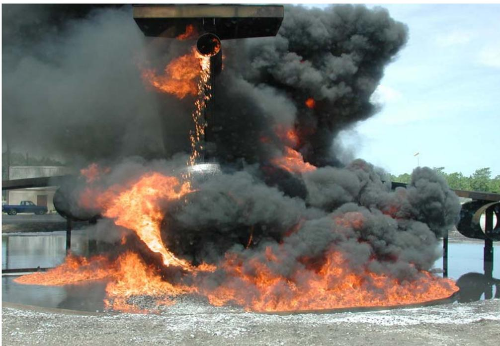
FIGURE 7. TAIL-MOUNTED, HIGH ENGINE NACELLE FIRE TEST DEVICE
