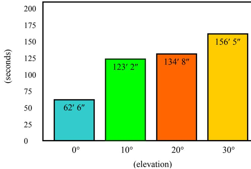
FIGURE 23. THE P-19 ROOF-MOUNTED TURRET AGENT STREAM THROW RANGE TESTS AT VARIOUS DEGREES OF ELEVATION
