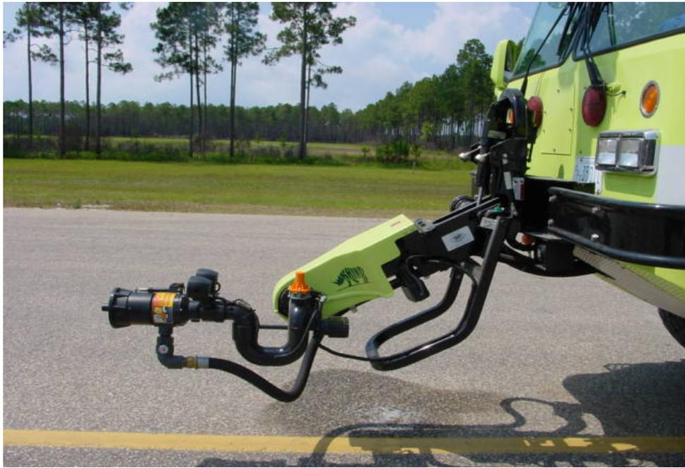
FIGURE 3. THE HPRV WITH 500-gpm HIGH-PERFORMANCE, MULTIPOSITION, BUMPER-MOUNTED TURRET
