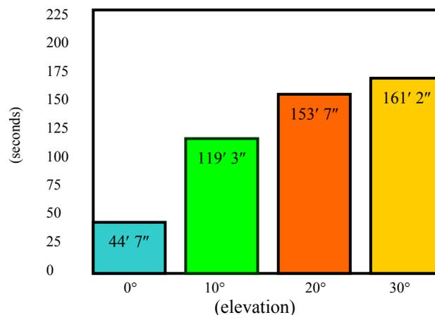
FIGURE 19a. THE HIGH-PERFORMANCE, MULTIPOSITION, BUMPER-MOUNTED TURRET WATER STREAM THROW RANGE TESTS, SET TO DIF POSITION AT VARIOUS DEGREES OF ELEVATION
