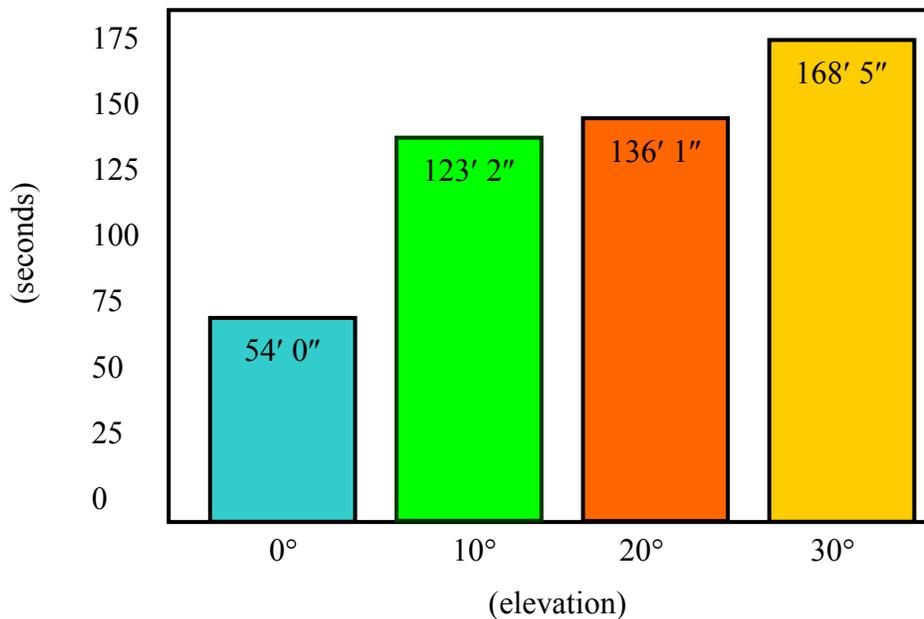
FIGURE 20. THE P-19 ROOF-MOUNTED TURRET WATER STREAM THROW RANGE TESTS AT VARIOUS DEGREES OF ELEVATION
