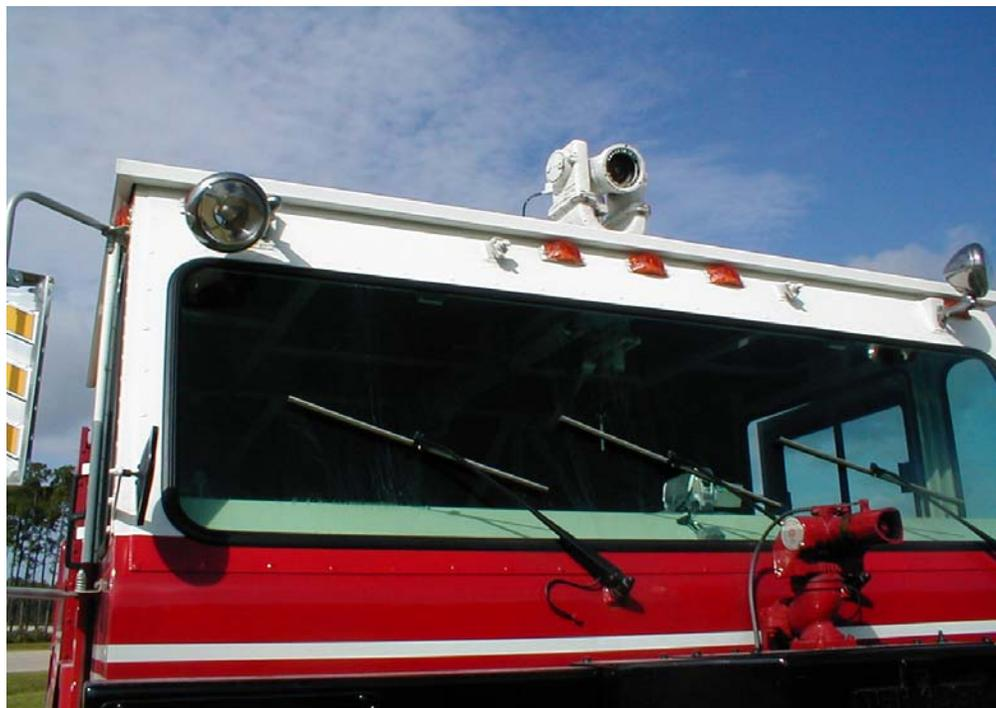
FIGURE 4. THE P-19 WITH A STANDARD 500-gpm ROOF-MOUNTED TURRET
