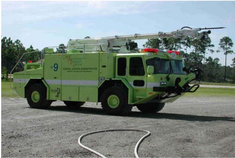
FIGURE 1. HIGH-PERFORMANCE RESEARCH VEHICLE WITH BUMPER-MOUNTED TURRET
