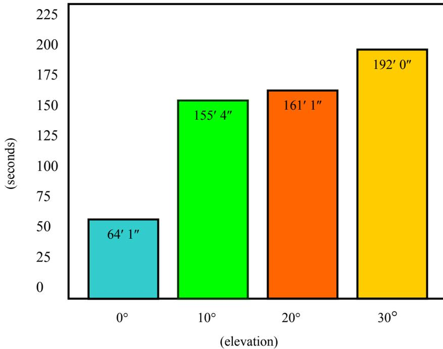
FIGURE 19b. THE HIGH-PERFORMANCE, MULTIPOSITION, BUMPER-MOUNTED TURRET WATER STREAM THROW RANGE TESTS, SET TO FULLY EXTENDED POSITION AT VARIOUS DEGREES OF ELEVATION
