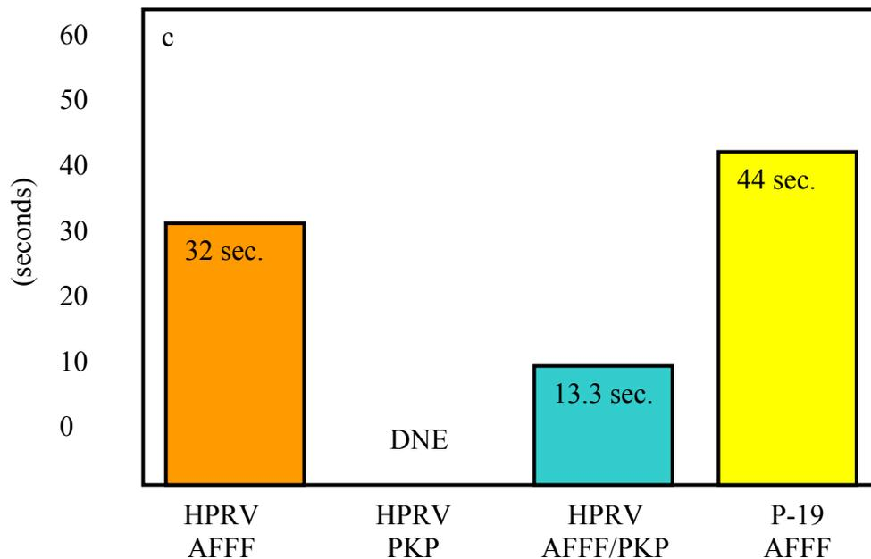
FIGURE 12. AVERAGE RESULTS OF THE F-100 ENGINE NACELLE FIRE TESTS
