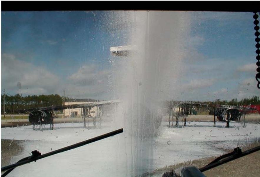
FIGURE 17. THE P-19 ROOF-MOUNTED TURRET USING AFFF
