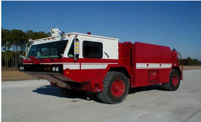
FIGURE 2. UNITED STATES AIR FORCE P-19 WITH ROOF-MOUNTED TURRET
