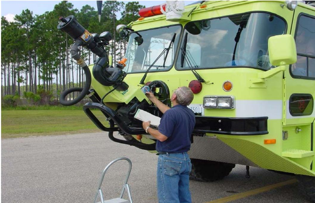
FIGURE 9. THE HIGH-PERFORMANCE, MULTIPOSITION, BUMPER-MOUNTED TURRET FULL-UP POSITION WITH THE TURRET AT 30°
