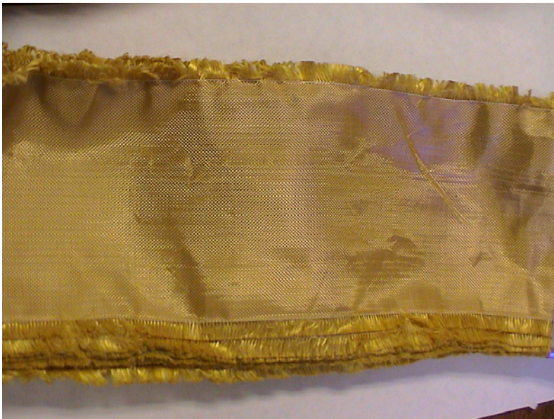
FIGURE A-30. FORMATION OF 2" WIDE BAND VISIBLE ALONG THE EDGE OF THE NOSE THROUGHOUT THE CIRCUMFERENCE (Zring24_1)
