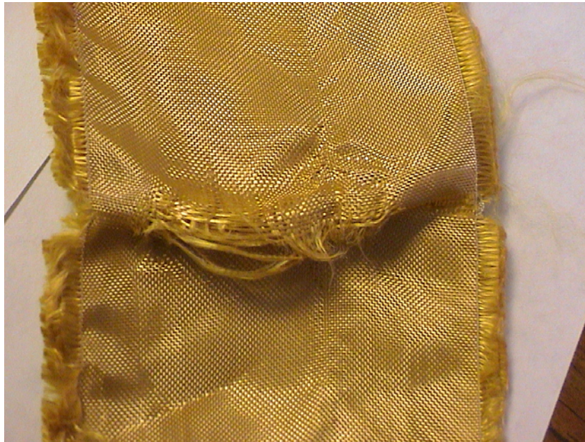
FIGURE A-20. COMPLETE NOSE PENETRATION (Zring2_1)
