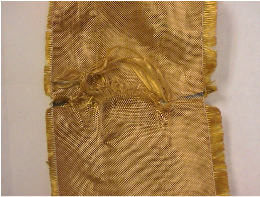
FIGURE A-17. COMPLETE NOSE PENETRATION (Zring1_2)
