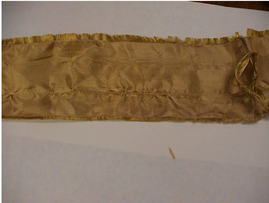
FIGURE A-18. YARN PULLOUT ALONG THE CIRCUMFERENCE AT THE EDGE OF THE NOSE (Zring1_2)
