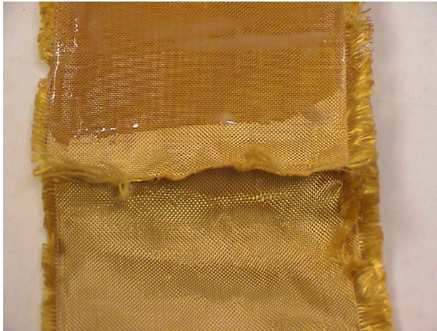
FIGURE A-21. OVERLAP PEEL-OFF (Zring2_1)
