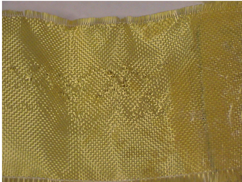
FIGURE A-3. REMOTE FAILURE AT THE CLAMP POSITION (Kring1_5)
