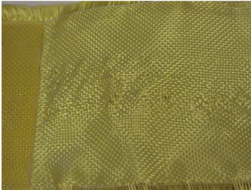
FIGURE A-9. REMOTE FAILURE AT CLAMP POSITION (Kring4_1)
