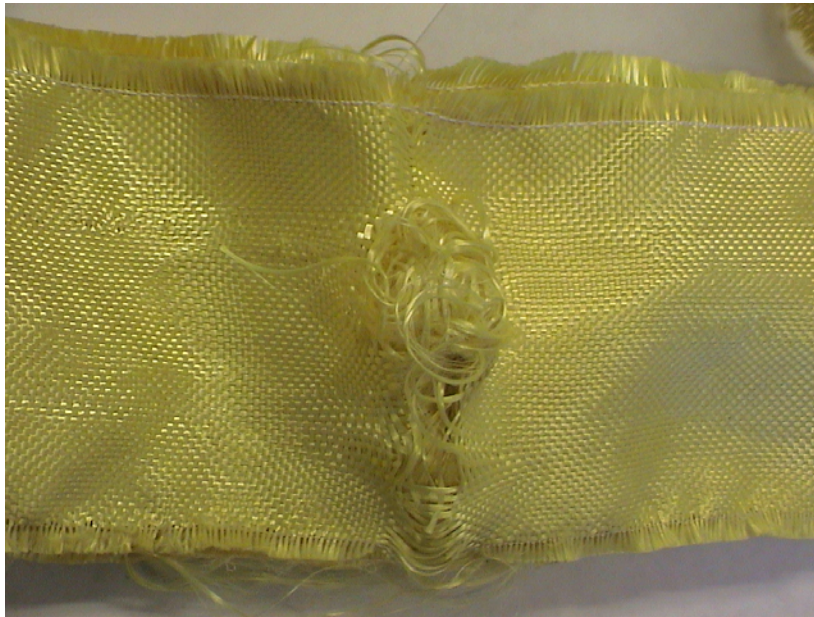
FIGURE A-11. FAILURE AROUND THE BLUNT NOSE CONTACT POINT, PARTIAL PENETRATION OF NOSE AT THE TOP (Kring8_1)
