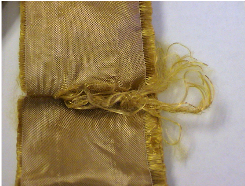
FIGURE A-23. COMPLETE NOSE PENETRATION (Zring4_2)
