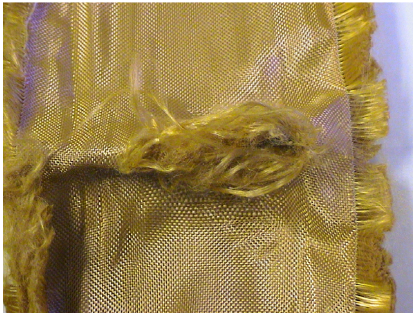
FIGURE A-26. COMPLETE NOSE PENETRATION (Zring8_3)
