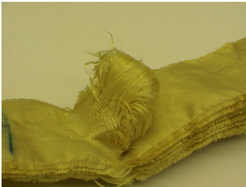
FIGURE A-14. FAILURE AROUND THE BLUNT NOSE CONTACT POINT PARTIAL PENETRATION OF NOSE AT THE TOP (Kring24_2)
