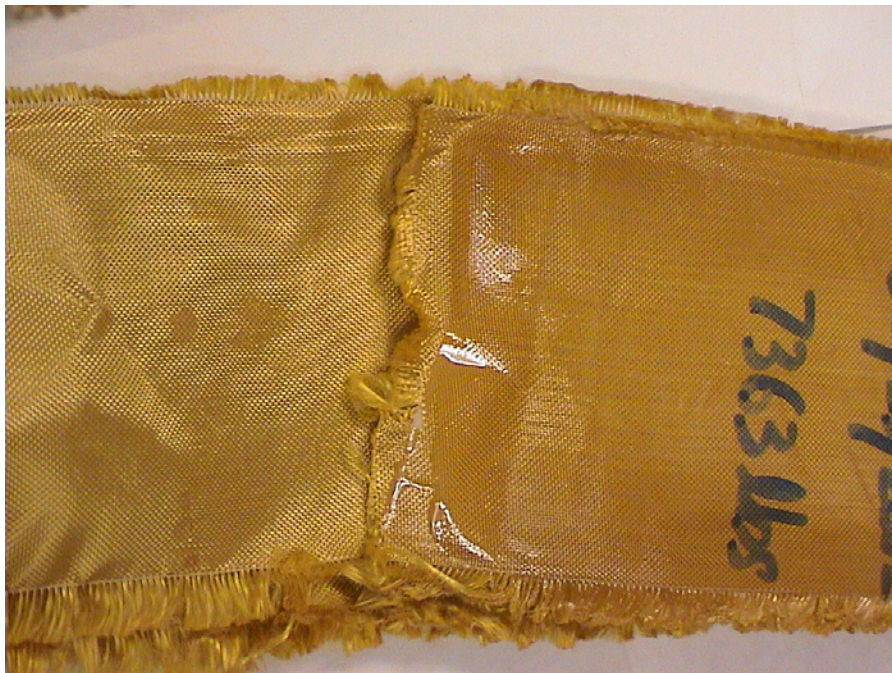
FIGURE A-24. OVERLAP PEEL-OFF (Zring4_2)
