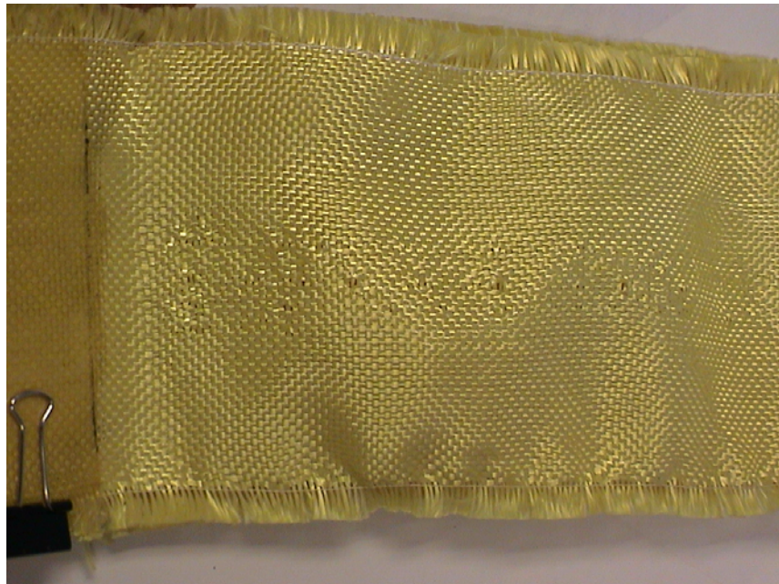
FIGURE A-6. REMOTE FAILURE AT CLAMP POSITION (Kring2_1)
