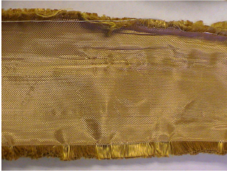
FIGURE A-27. FORMATION OF 2" WIDE BAND VISIBLE ALONG THE EDGE OF THE NOSE THROUGHOUT THE CIRCUMFERENCE (Zring8_3)
