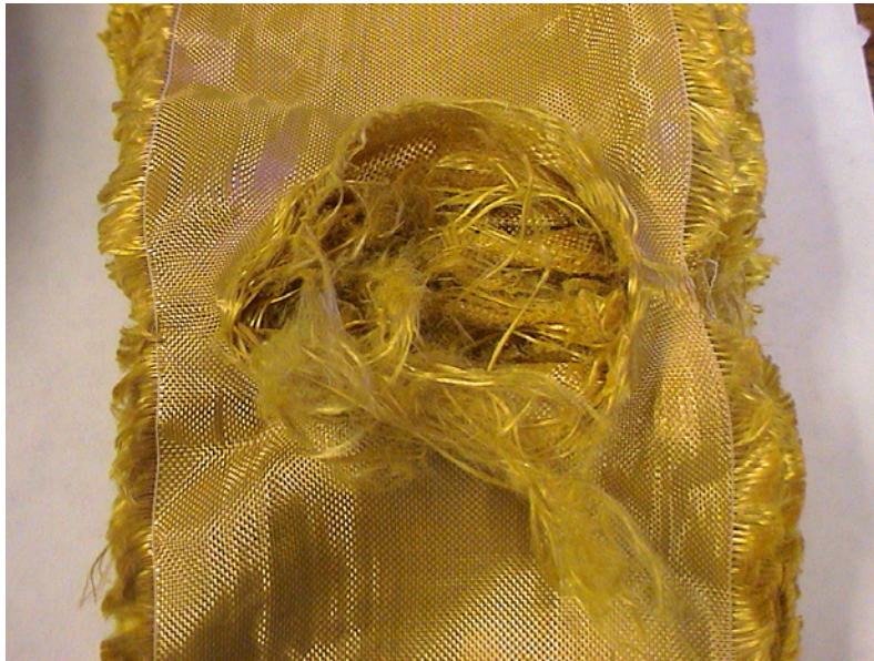
FIGURE A-29. COMPLETE NOSE PENETRATION (Zring24_1)
