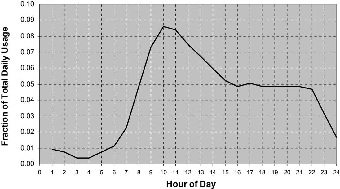
**Figure 6. Clothes washer hot water use profile**
