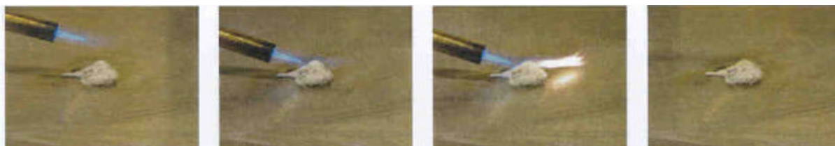
Figure 2. Flame test with LiH slurry.
