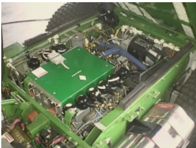
Figure 8. NG2000™, 8 kW, installed in Deere & Co. Gator™ industrial vehicle.
