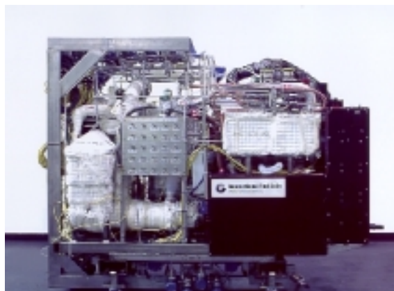
IFC 50-kW gasoline-fueled, PEM fuel cell power plant ready for verification testing.
