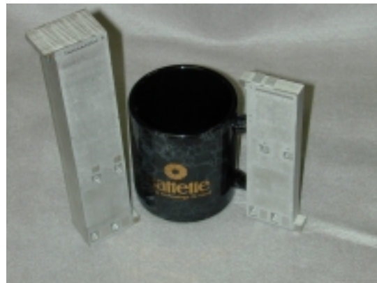
Figure 3. Integrated multistream microchannel heat exchangers prior to header attachment. Unit on left contains a combustion gas recuperator and water vaporizer. Unit on right contains a 90%-effective reformate recuperator, a fuel vaporizer, and a water preheater. These two units are designed to support up to a maximum of a 5-kW e steam reformer operating a 3:1 steam-to-carbon ratio.
