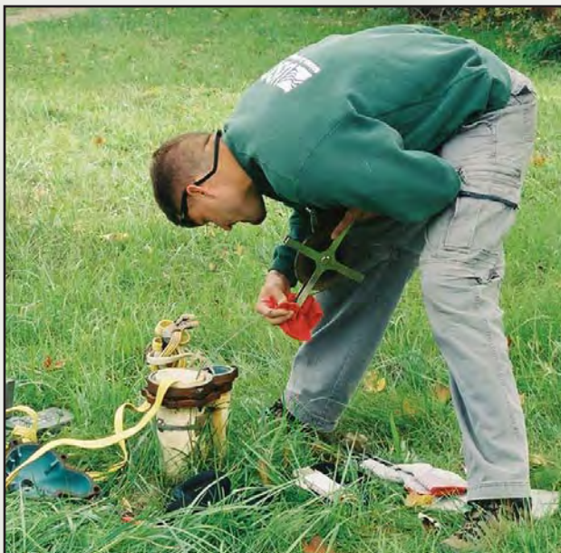
Figure 4. Measurements of water levels in ground-water wells are needed to define the direction of groundwater flow.
