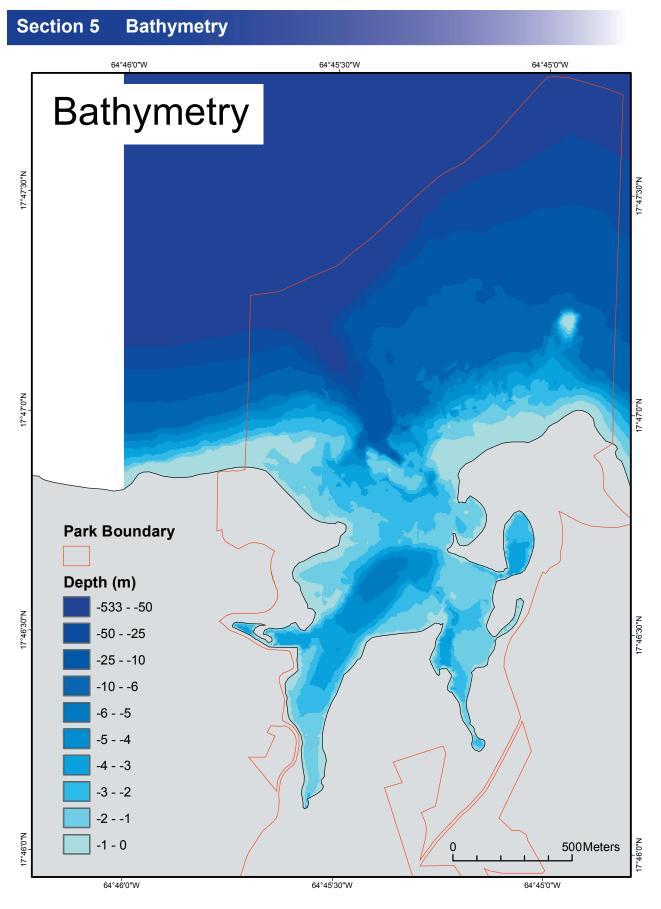
**Figure 5.1.** Interpolated bathymetry for SARI, based on the available soundings conducted in 1982 and 1977 from NOAA Geophysical Data System (GEODAS).
