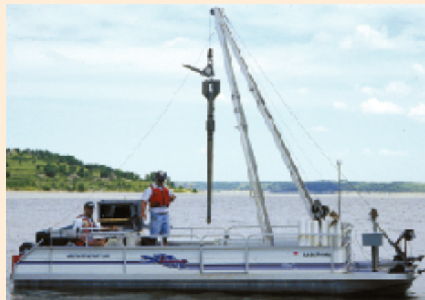
Figure 1. Bottom-sediment cores were collected with a gravity corer mounted on a pontoon boat. The corer is lowered to a designated distance above the sediment and allowed to free fall to penetrate through the entire thickness of reservoir bottom sediment.
