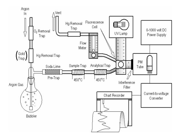
**Figure 2.** Schematic Diagram of the Cold Vapor Atomic Fluorescence Spectrometer (CVAFS) System
