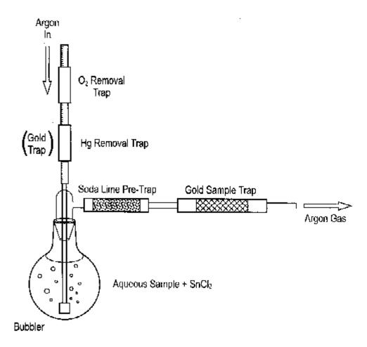
Figure 1. Schematic Diagram of Bubbler Setup
