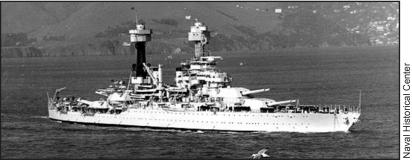
Figure 31. USS *West Virginia*, BB-48, Colorado class. Completed in 1923. Displacement: 33,590 tons Maximum speed: 21 knots Crew: 1,626 Armament: eight 16-inch guns, 26 5-inch guns
