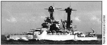
Figure 28. USS *Tennessee*, BB-43, Tennessee class. Completed in 1920. Displacement: 33,100 tons Maximum speed: 21 knots Crew: 1,625 Armament: 12 14-inch guns, 16 5-inch guns
