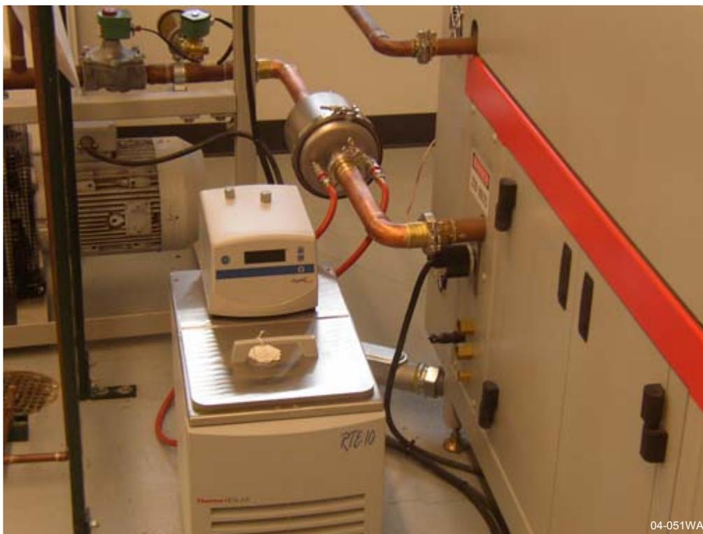
**Figure 30 Cold trap and chiller installed on laminator vacuum system.**
