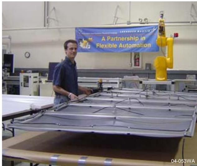
**Figure 34 Tedlar sheet (5' x 12') lifted by a vacuum end effector.**
