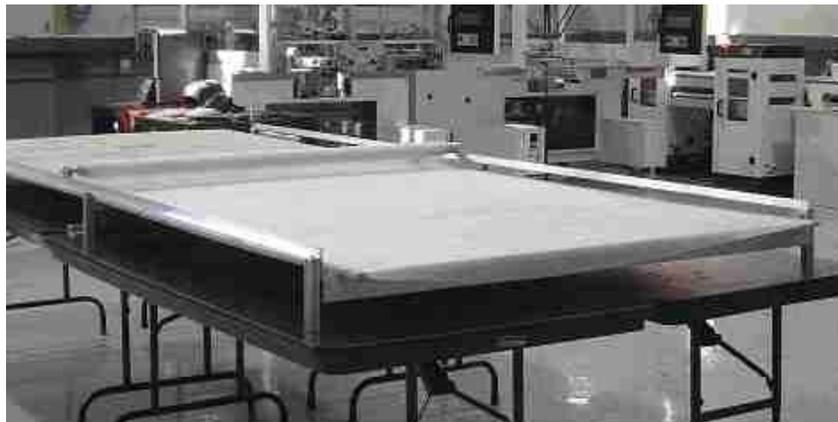
**Figure 36** Prototype sheet unroller.
