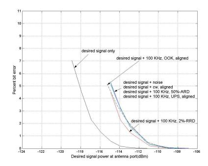
Figure 4.8. Percent bit-error versus variable LMR power for Receiver B in P25 mode – 100-kHz PRF UWB interference.
