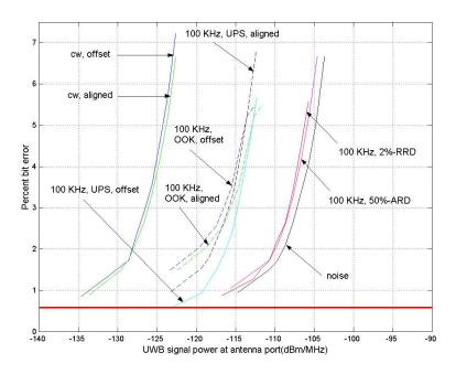
Figure 4.6. Percent bit-error versus variable interference power density for Receiver B in P25 mode – 100-kHz PRF UWB interference.
