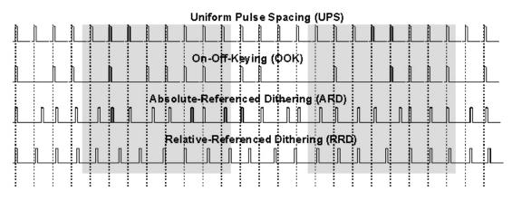
Figure 2.1. Pulse spacing modes.
