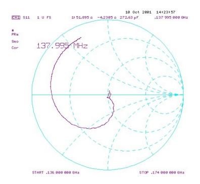
Figure 3.5. Input impedance to receiver B as seen at the input to the matching stub.
