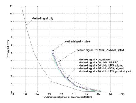
Figure 4.5. Percent bit-error versus variable LMR power for Receiver A in P25 mode – 20-MHz PRF UWB interference.
