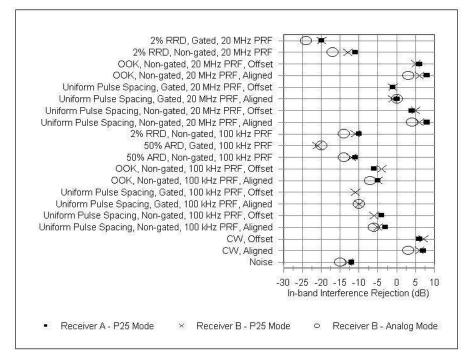
Figure 4.1. In-band interference rejection ( $P_{REF} - P_I$ ).
