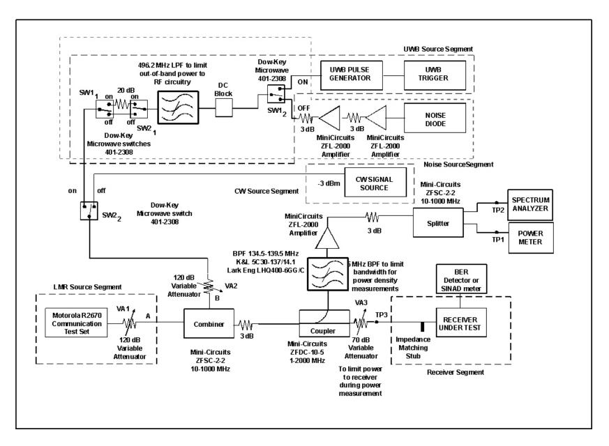
Figure 3.2. Block diagram of measurement system.
