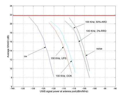
Figure 4.10. Average SINAD versus variable interference power density for Receiver B in analog mode – 100-kHz PRF UWB interference.
