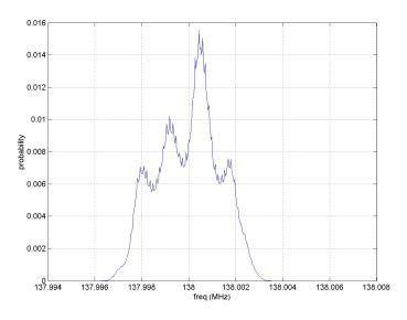
Figure 3.3. Frequency histogram of the C4FM modulated signal.
