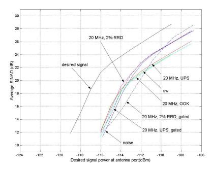
Figure 4.13. Average SINAD versus variable LMR power for Receiver B in analog mode – 20-MHz PRF UWB interference.
