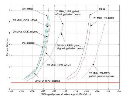
Figure 4.7. Percent bit-error versus variable interference power density for Receiver A in P25 mode – 20-MHz PRF UWB interference.
