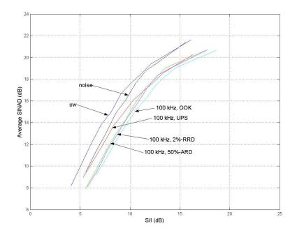
Figure 4.18. Average SINAD versus S/I for Receiver B in analog mode – 100-kHz PRF UWB interference.
