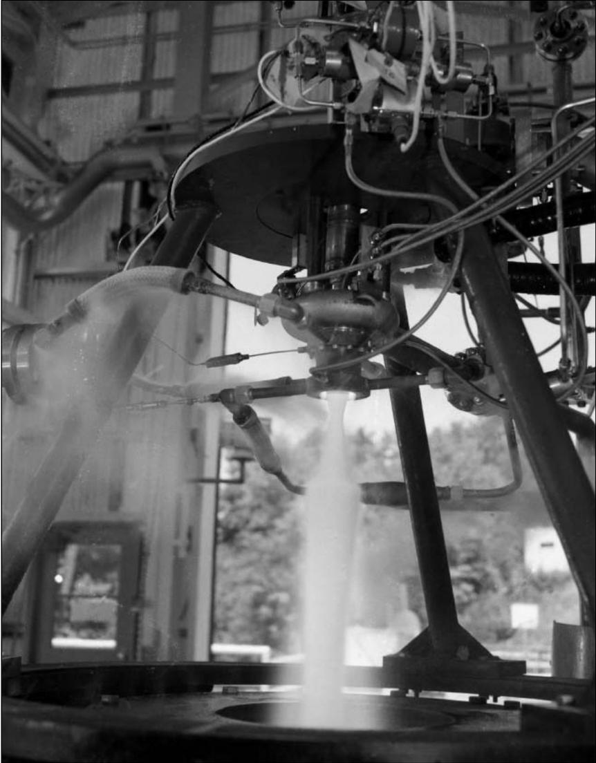
Test of a 5,000-pound-thrust engine used to investigate low cycle thermal fatigue, 4 October 1975.
