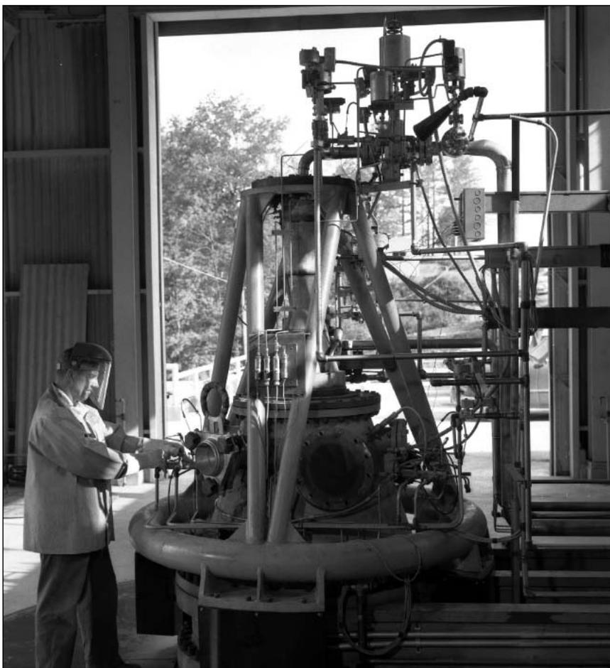
A technician checks the installation of the 20,000-pound-thrust rocket engine on the test stand, October 1957.
