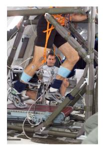
Figure 3. Close-up of connection between harness and loading bungee illustrating load cell orientation during data collection.
