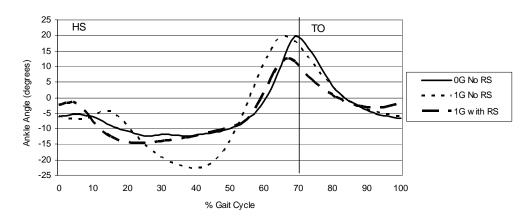
Figure 10. Typical lower extremity joint kinematics for locomotion on the BD-1 at  $5 \text{ km} \cdot h^{-1}$ . HS = Heel Strike and TO = Toe Off.
