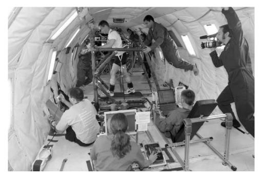
Figure 2. BD-1 treadmill evaluation experiment being performed on NASA KC-135 Research Aircraft.
