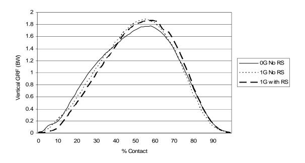
Figure 8. Typical vertical GRF trajectory during 8 km·h<sup>-1</sup> locomotion in 0G and 1G on BD-1.
