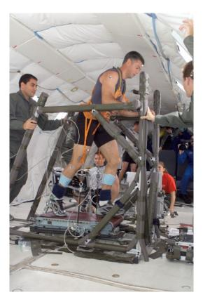
Figure 1. The BD-1 treadmill. The padded frame surrounding the subject was used for safety purposes and to provide a handrail that subjects could push against; it is not a part of the treadmill.
