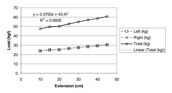
Figure 5. Bungee load versus extension calibration curve. The lower curves represent the load and extension measured on each side. The upper curve is the sum of these two curves, representing the overall bungee system load versus extension curve.
