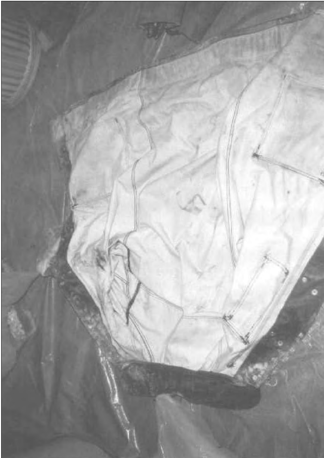
Photo by J. Gordon Routley Coat worn without thermal liner was burned through in only a small area of the right arm pit. The firefighter wearing this coat would have been very critically burned if the amount of sodium splashed on the outer shell had been greater.
