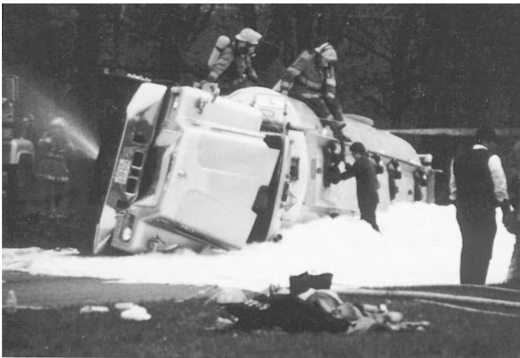
5. Contractor personnel complete off-loading operation. Firefighters atop tank are at position of hole that was drilled. Note water spray directed at exhaust pipe of the recovery tanker.
