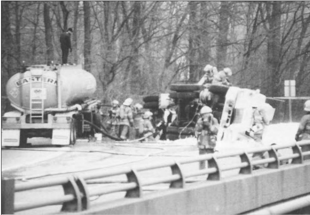
4. Second tanker pumping fuel from the overturned tanker.
