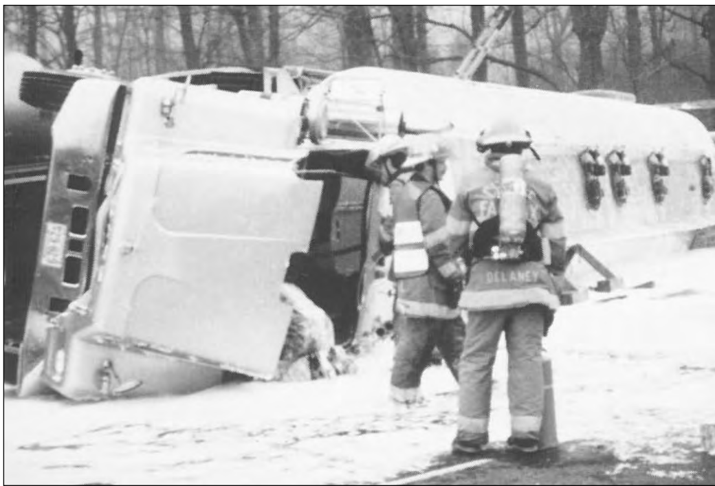
1. Overturned tanker showing dome covers.
