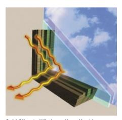
**Cold Climate Windows Keep Heat In**Double-pane windows with low-e coating on the glass reflect heat back into the room during the winter months.
