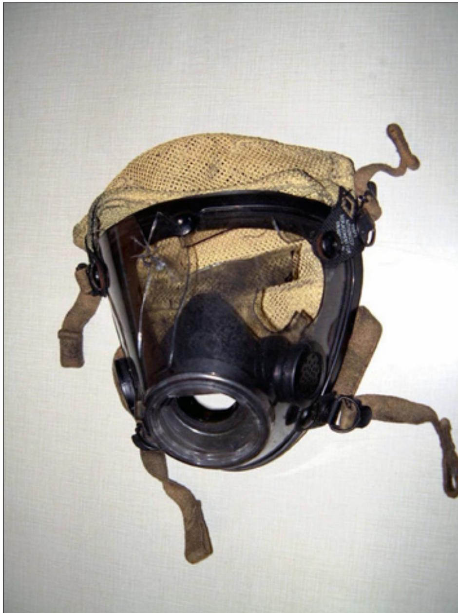
**#49** Faceshield on SCBA cracked by flying debris from explosion
