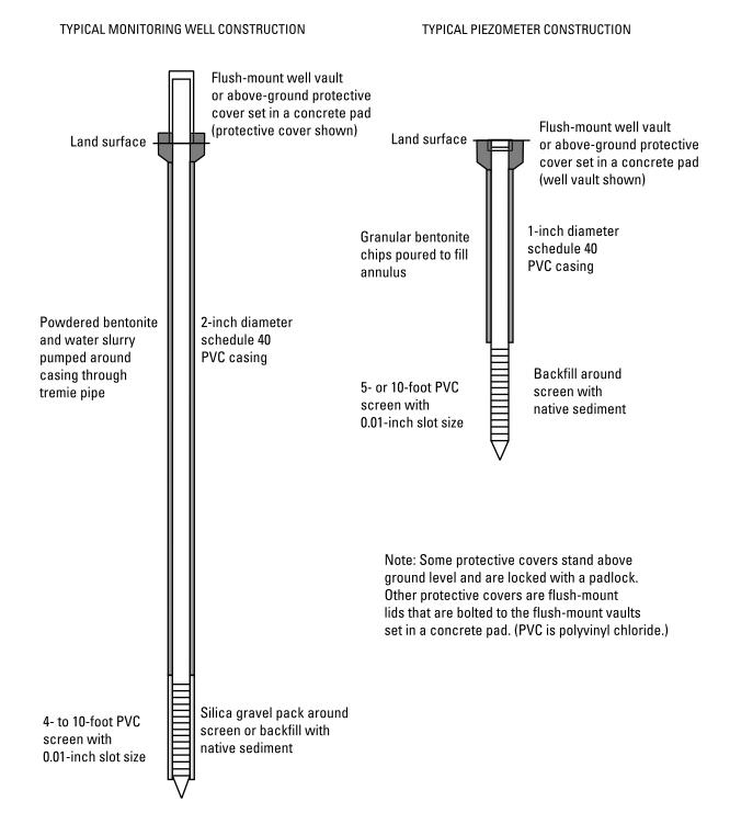
**Figure 6.** Diagram of monitoring wells and piezometers for investigation of the hydrogeologic framework in Quaternary deposits at the U.S. Army Atterbury Joint Maneuver Training Center near Edinburgh, Indiana.
