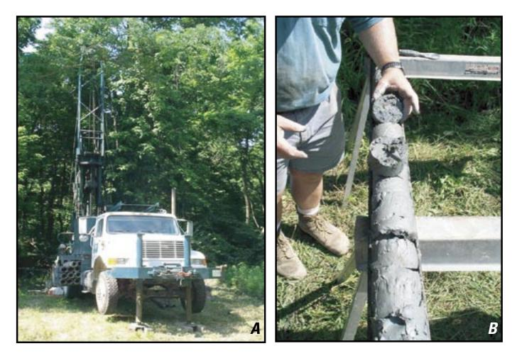
Figure 4. Photographs of (A) the truck-mounted hollow-stem auger drill rig used to collect sediment cores and construct monitoring wells and (B) an example core collected with this drill rig at the U.S. Army Atterbury Joint Maneuver Training Center, near Edinburgh, Indiana.
