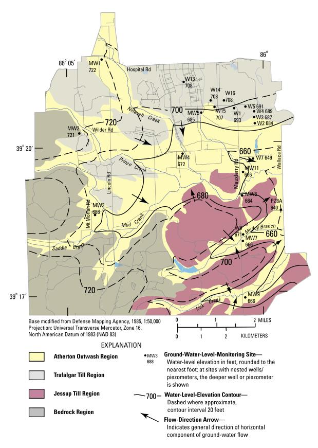
**Figure 11.** Ground-water elevations at selected monitoring locations, generalized ground-water elevation contours, and generalized directions of horizontal ground-water flow on July 31 and August 1, 2003, in the hydrogeologic-framework study area at the U.S. Army Atterbury Joint Maneuver Training Center near Edinburgh, Indiana.
