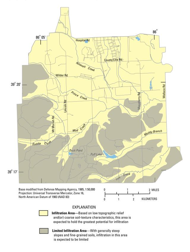
**Figure 10.** Infiltration areas determined by low topographic relief and(or) coarse-grained soil texture in the hydrogeologic-framework study area at the U.S. Army Atterbury Joint Maneuver Training Center near Edinburgh, Indiana.
