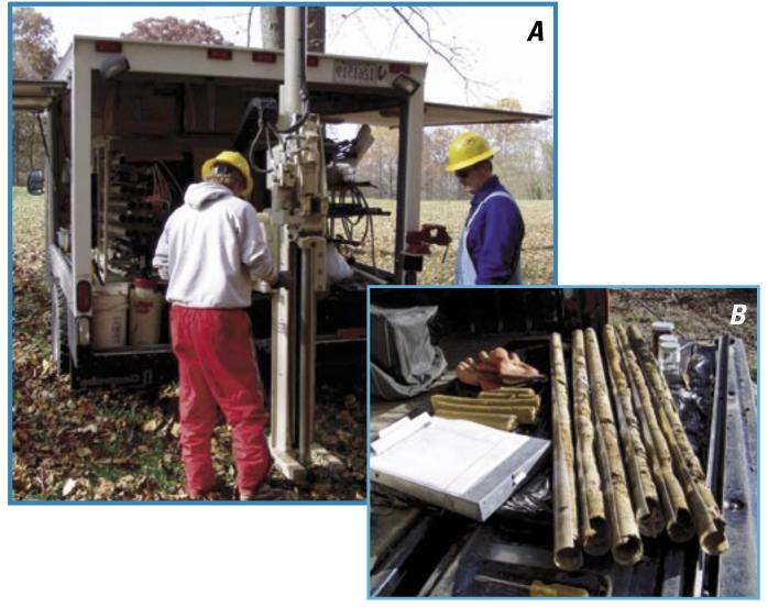
**Figure 5.** Photographs of (A) the direct-push drill rig used to collect sediment cores and construct piezometers at the U.S. Army Atterbury Joint Maneuver Training Center, near Edinburgh, Indiana, and (B) a core collected with this drill rig.
