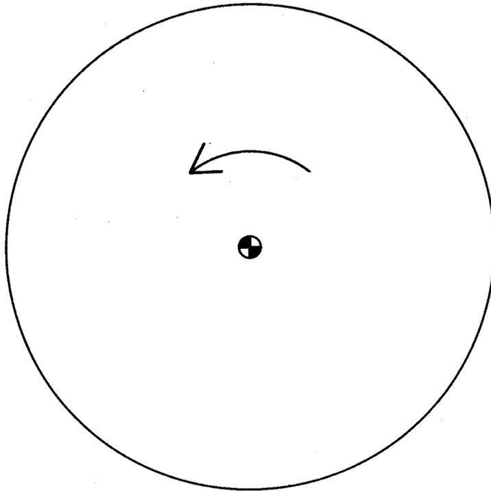
To fly a ground track which is a perfect circle around the pylon, remaining at all times the same distance from the pylon, the angle of bank will have to be varied when there is a wind.
