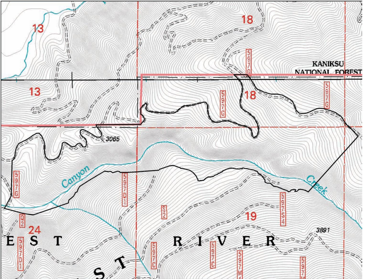
**Figure 4**—Elevation contour lines for Wellner Cliffs RNA. Lines show 5-meter contours generated from a 10-meter digital elevation model.
