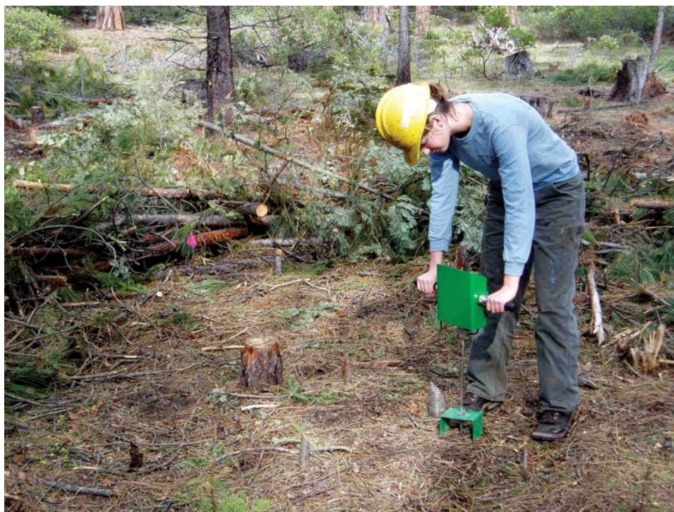
Measuring soil resistance using the recording soil penetrometer.
