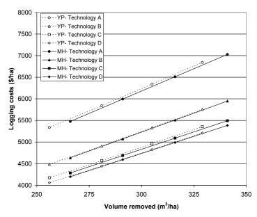
Figure 3.—Logging costs by volume removed for mixed hardwood and yellow-poplar stands for four different logging systems (see Table 3 and Page 3 for description of technologies used).
