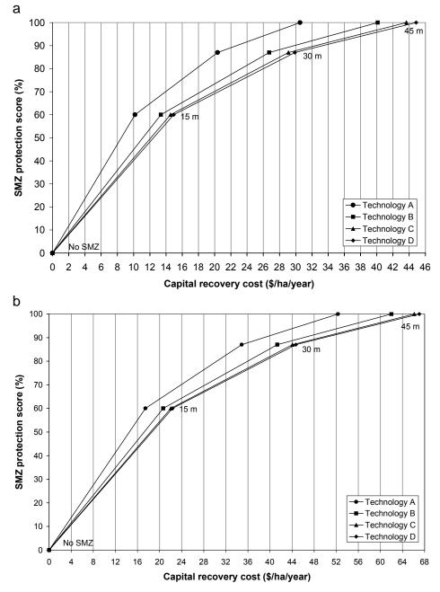
Figure 6.—SMZ protection scores compared with capital recovery costs for the (a) yellowpoplar and (b) mixed hardwood stands under the four harvesting technologies. Symbols and lines represent different logging systems. SMZ protection scores are labeled on corresponding SMZ width (See Table 3 and Page 3 for description of technologies used).
