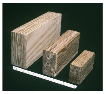
Figure 1. Examples of types of composite lumber products tested in this study: (left to right) laminated veneer lumber, parallel strand lumber, and laminated strand lumber.
