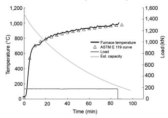
Figure 27. Furnace temperature, applied load, and estimated residual load capacity in tension test of Douglasfir laminated veneer lumber (Test Number 8).
