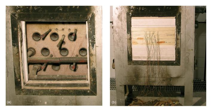
Figure 2. Opening of small vertical furnace (a) without and (b) with a test specimen in place.
