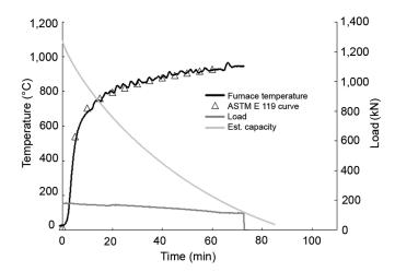
Figure 22. Furnace temperature, applied load, and estimated residual load capacity in tension test of Douglasfir laminated veneer lumber (Test Number 3).
