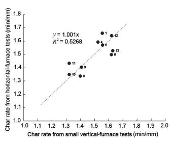
Figure 18. For the different materials, comparison of charring rates ( $m_1$ ) obtained in the horizontal-furnace tests with those obtained in the small vertical-furnace tests. Labels are the material numbers listed in Table 1.
