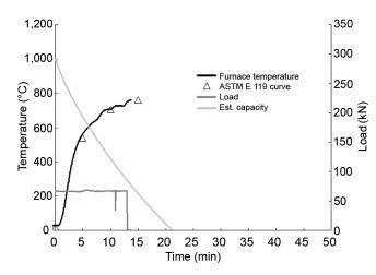
Figure 21. Furnace temperature, applied load, and estimated residual load capacity in tension test of aspen laminated veneer lumber (Test Number 2).
