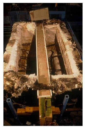
Figure 6. Unloaded specimen in horizontal-furnace test.
