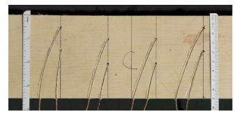
Figure 3. Location of thermocouples in one of the laminates that was glued together to make the specimen for small vertical-furnace tests. With thermocouples in three laminates, a total of six thermocouples was at each of the four distances (13, 25, 38, and 51 mm) from the fireexposed surface.
