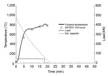
Figure 29. Furnace temperature, applied load, and estimated residual load capacity in tension test of Southern Pine laminated veneer lumber (Test Number 10).
