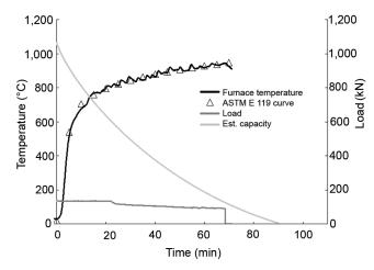
Figure 26. Furnace temperature, applied load, and estimated residual load capacity in tension test of Douglasfir laminated veneer lumber (Test Number 7).
