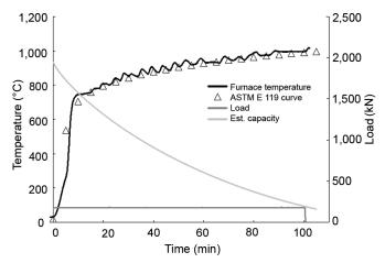
Figure 32. Furnace temperature, applied load, and estimated residual load capacity in tension test of Douglasfir PSL (Test Number 13).
