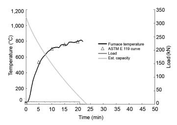
Figure 24. Furnace temperature, applied load, and estimated residual load capacity in tension test of Douglasfir laminated veneer lumber (Test Number 5).
