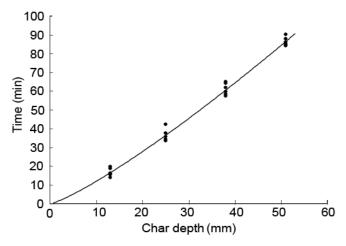
Figure 4. Example of the time–location data for one small vertical-furnace test. The data were obtained from 24 thermocouples located at different depths in a specimen. The curve is a power function.
