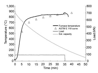
Figure 20. Furnace temperature, applied load, and estimated residual load capacity in tension test of yellowpoplar LSL (Test Number 1).
