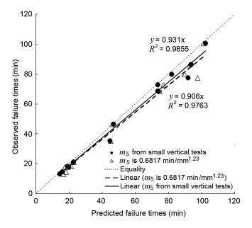
Figure 33. Comparison of the experimental observed failure times for the tension specimens with the predicted failure times from the TR 10 methodology.
