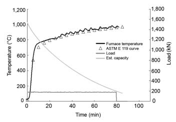
Figure 30. Furnace temperature, applied load, and estimated residual load capacity in tension test of Southern Pine laminated veneer lumber (Test Number 11).
