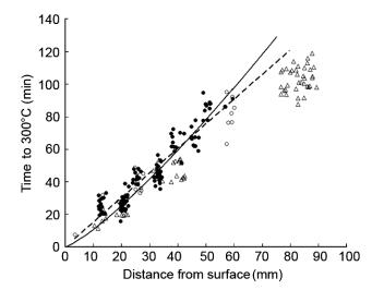
Figure 7. Plot of experimental data (symbols) and predictions based on  $x_c$  model (- -) and  $x_c^{1.23}$  model (---) of data. Solid circles (•) are for locations greater than 13 mm from horizontal center of test specimen. Open circles ( $\circ$ ) are data for locations between 13 and 30 mm from the horizontal center of the test specimen. Open triangles ( $\Delta$ ) are locations less than 13 mm from the center of the test specimen.
