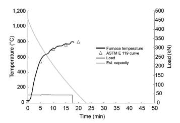
Figure 28. Furnace temperature, applied load, and estimated residual load capacity in tension test of eucalyptus laminated veneer lumber (Test Number 9).
