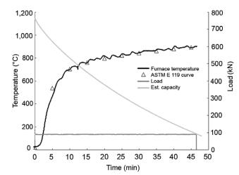
Figure 25. Furnace temperature, applied load, and estimated residual load capacity in tension test of Douglasfir laminated veneer lumber (Test Number 6).
