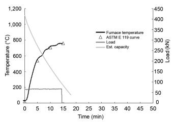
Figure 31. Furnace temperature, applied load, and estimated residual load capacity in tension test of yellowpoplar laminated veneer lumber (Test Number 12).
