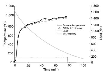
Figure 23. Furnace temperature, applied load, and estimated residual load capacity in tension test of Douglasfir laminated veneer lumber (Test Number 4).
