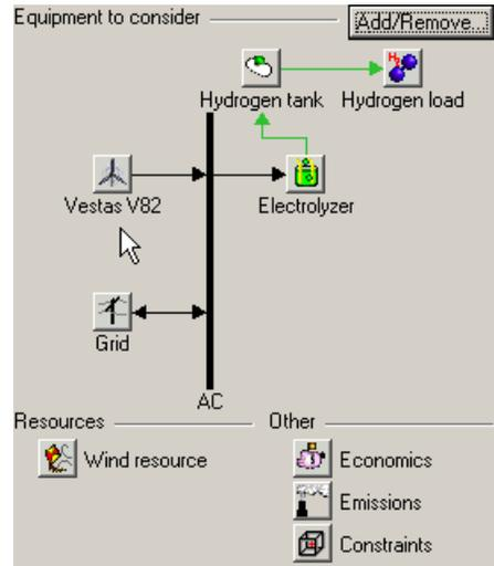
**Figure 3: System Components for Case 1 in the Model**
