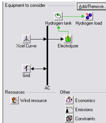
**Figure 5: System Components for Case 2 in the Model**
