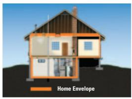
The exterior of your home is called the "envelope" or "shell". (See the orange line showing the envelope in the diagram above.) The envelope is made up of the outer walls, ceiling, windows and floor. Improving your envelope can make your home more comfortable, especially under extremely hot or cold conditions, and help lower your energy bills.
