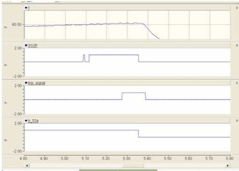
Figure 7. 60.5 Hz overfrequency
