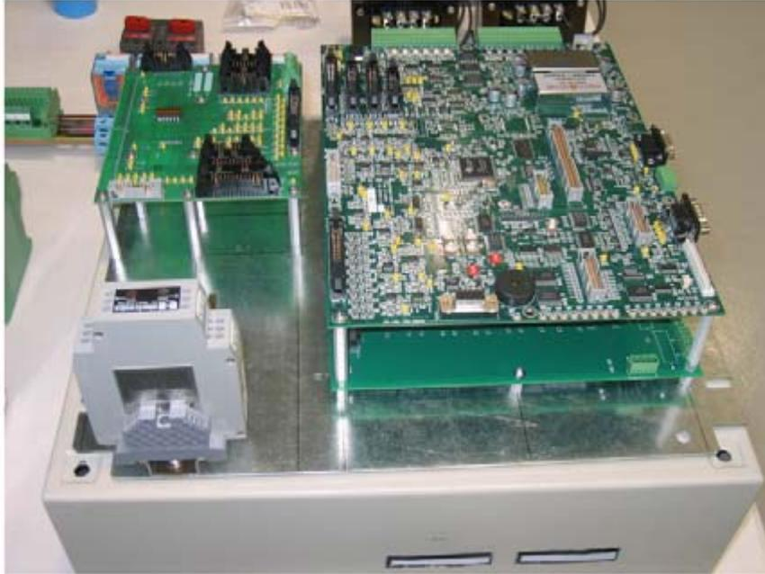
Figure 33. DER Switch controller
