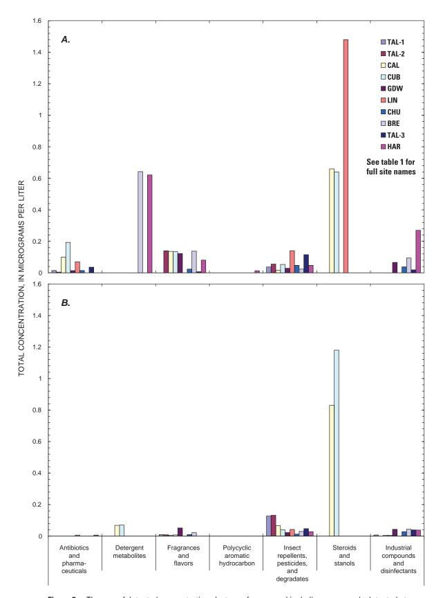
**Figure 5.** The sum of detected concentrations by type of compound including compounds detected at concentrations above the laboratory reporting level and estimated below the laboratory reporting level from samples collected during (*A*) a high base-flow period in April and (*B*) a low base-flow period in October in the lower Tallapoosa River watershed, Alabama, 2005.
