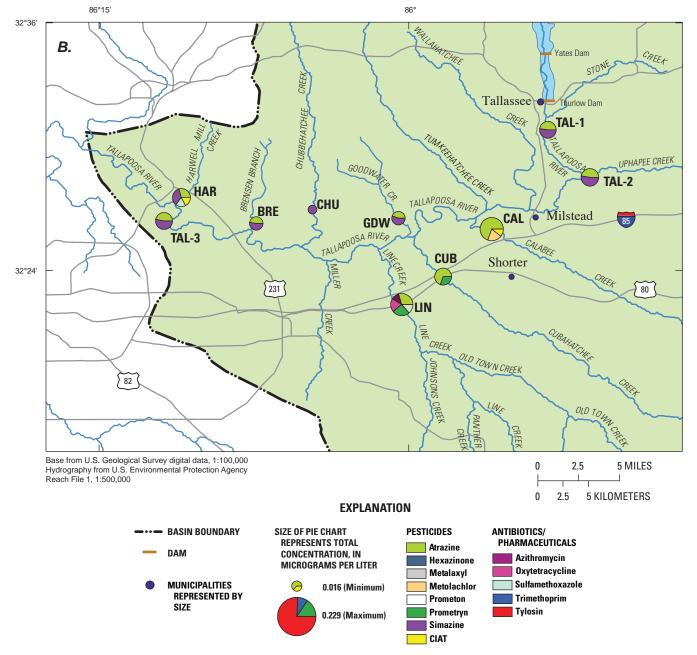
**Figure 4.** Total concentrations of all compounds detected above and below the laboratory reporting level in samples collected during (*A*) a high base-flow period in April and (*B*) a low base-flow period in October in the lower Tallapoosa River watershed, Alabama, 2005.—Continued
