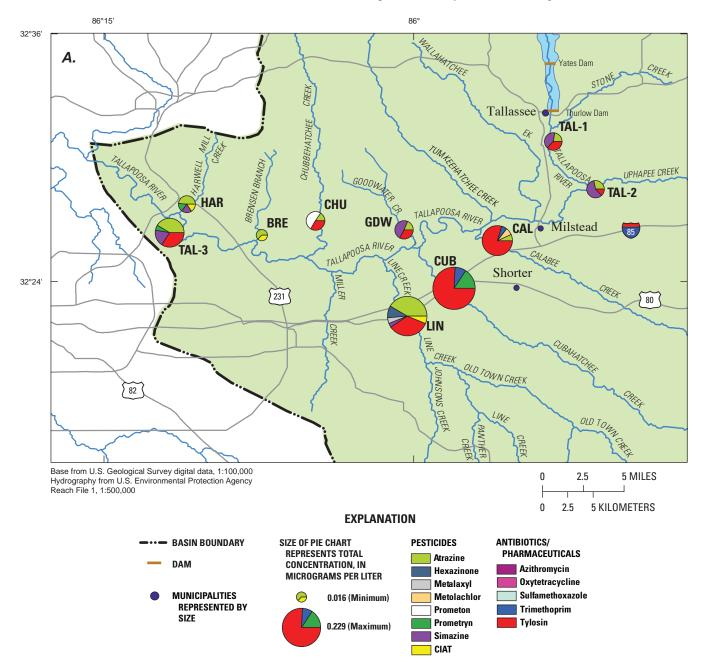
**Figure 4.** Total concentrations of all compounds detected above and below the laboratory reporting level in samples collected during (*A*) a high base-flow period in April and (*B*) a low base-flow period in October in the lower Tallapoosa River watershed, Alabama, 2005.
