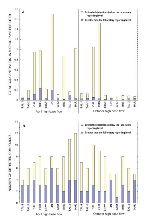
**Figure 3.** Summary of compounds detected in concentrations greater than the laboratory reporting level and at estimated concentrations summarized by the (*A*) total concentration in the sample and (*B*) number of compounds in the sample collected from the lower Tallapoosa River watershed, Alabama, 2005.
