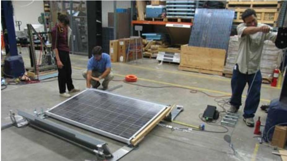
**Figure 39: Lateral load test on an RFT10 assembly. A tensile load is applied to the east side of the assembly.**
