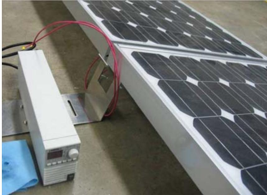
**Figure 42: Grounding test on an RFT10 assembly.**
