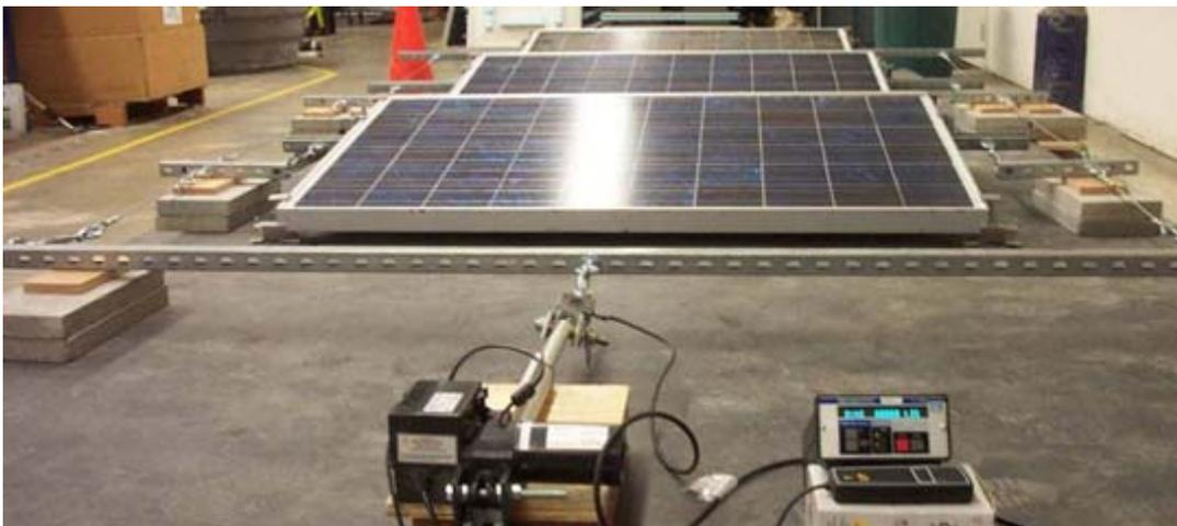
**Figure 43: Friction test on an RFT10 assembly.**
