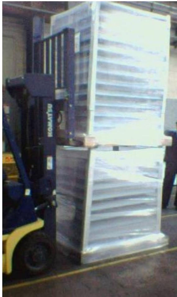
**Figure 54: Test of corner supports in double stacked pallets**
