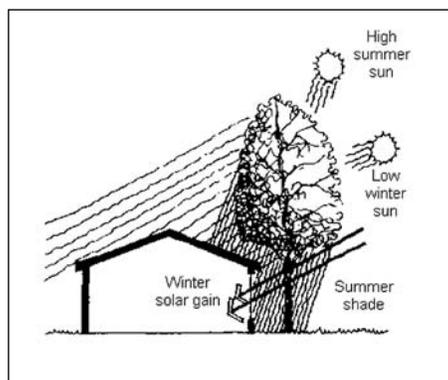
Figure 25—Select solar-friendly trees for southern exposures and locate them close enough to provide winter solar access and summer shade (from Sand 1991).
