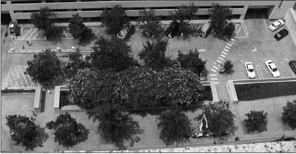
Figure 7—Trees planted to shade parking areas can reduce hydrocarbon emissions and improve air quality.
