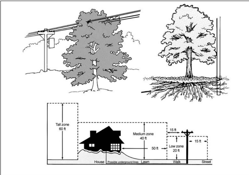
Figure 31—Know where power lines and other utility lines are before planting. Under power lines use only small-growing trees (“low zone”) and avoid planting directly above underground utilities. Larger trees may be planted where space permits (“medium” and “tall zones”) (from ISA 1992).
