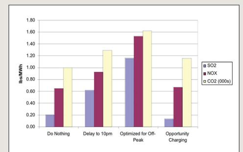
Figure 5. Upstream Emission Rates Impact of PHEVs (50k Vehicles)
