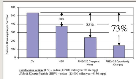
Figure 2. Comparative Fuel Consumption for PHEVs
