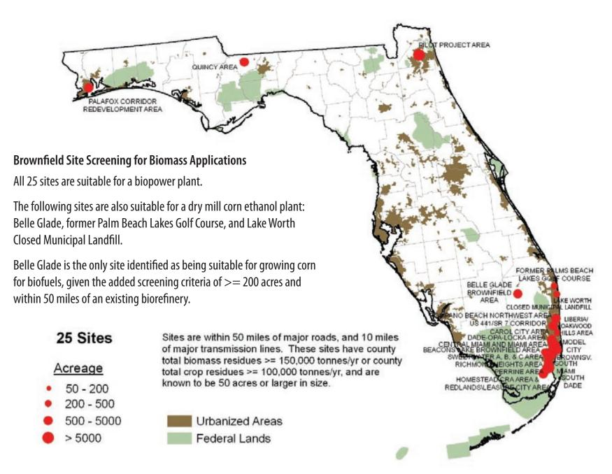
Figure 9. Identification of Suitable Sites for Biomass Applications
