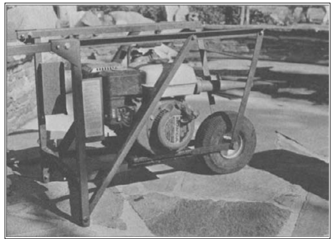
Figure 2 —Portable fire pump used by a homeowner to protect his residence with pool water and Class A foam concentrate.
