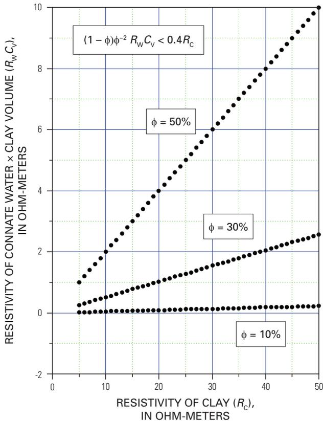
**Figure 3.** Graph showing relationship between the resistivity of clay ( $R_c$ ) and the product of connate-water resistivity ( $R_w$ ) and clay volume ( $C_v$ ) required to yield an approximate linear relationship between  $\log$  resistivity and  $\log$  porosity. The values under each curve satisfy the linearity condition.
