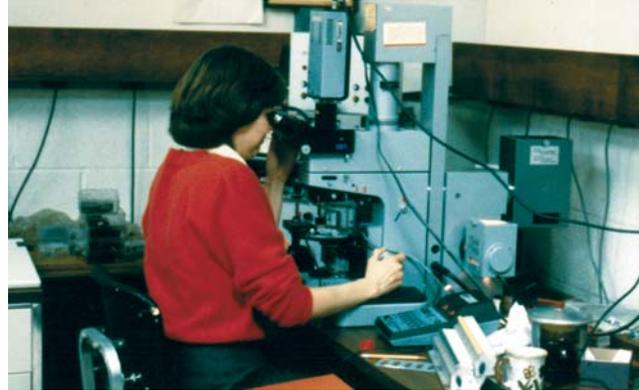
**Figure 28.** Photograph of a coal scientist at work identifying coal macerals and rank in a polished sample of coal using a high-powered, reflected-light microscope. Photograph by R.W. Stanton (U.S. Geological Survey).
