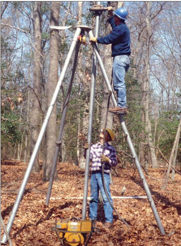
Tripod used to support aluminum pipe with vibrator on upper end.
