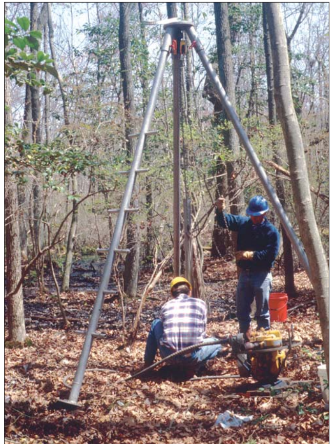
Extracting the core barrel from the ground using an automobile engine winch.
