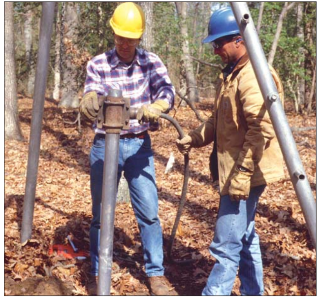
Core pipe was vibrated approximately 8 feet into the ground.
