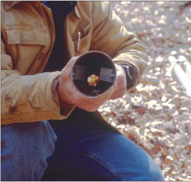
Flanges inside bottom of pipe to retain soft sediment core.
