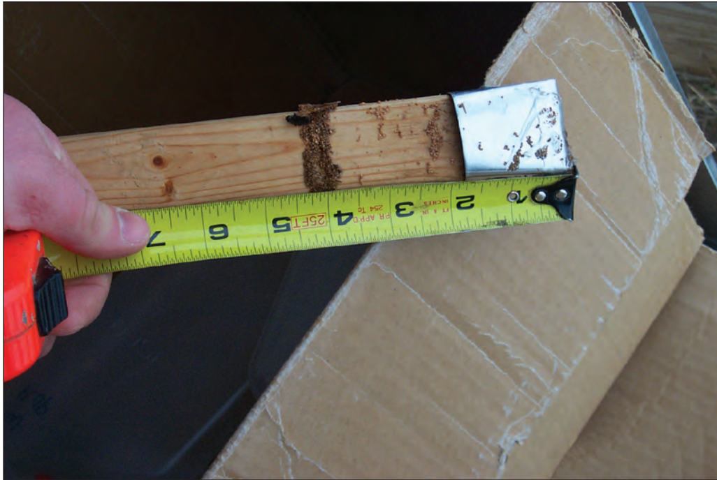
Figure 7. Measurements of the cork line on the crest-stage gages were made after a surface-water runoff event
