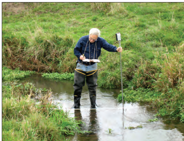
Figure 17. U.S. Geological Survey field technician making a discharge measurement at a streamgaging station at Pioneer Farm.
