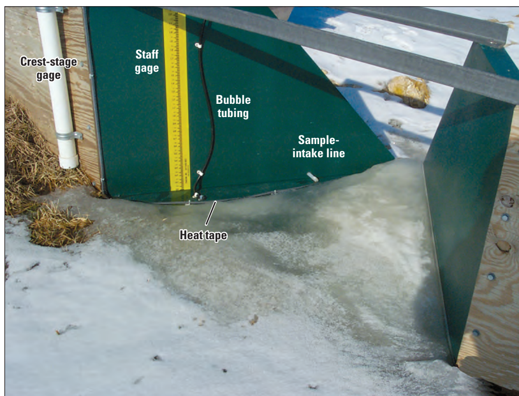
Figure 8. Ice was removed from H flumes before runoff events. Here, icemelt near the bubble line and sample-intake line due to the heat tape can be seen.
