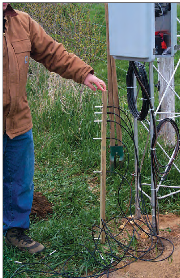
Figure 22. Soil-temperature probes ready for installation.
