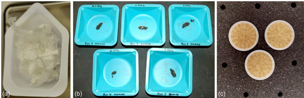
Figure 28.—Nomex fuel tests. (a) Nomex snips before heating (0.5 g fuel sample). (b) After heating, the Nomex snips became one or two compact pieces of char/ash, as shown in the remains of five different tests. (c) TEOM filters after mass concentration measurements of Nomex smoke particles show the characteristic yellowish color of brown carbon.
